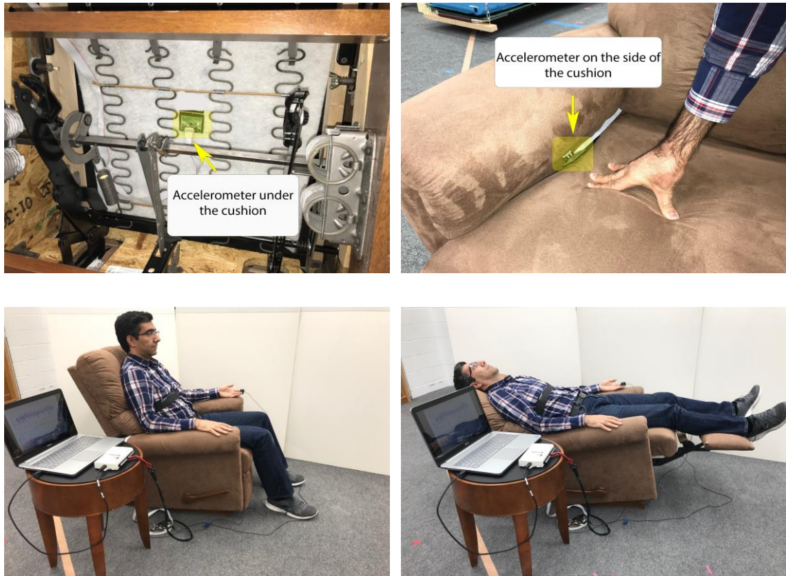
Figure 3.2. MU's accelerometer-based chair sensor for vital sign monitoring (a) Accelerometer placed under the seat cushion of the recliner chair. (b) Accelerometer placed on the side of the seat cushion, hidden between the seat cushion and the arm of the chair. The accelerometers are not visible during normal operation and require no contact with the occupant to function. (c,d) Two chair positions were tested in the study: Upright (left) and Reclined (right). For ground truth reference, a chest band and a finger pulse transducer were worn by each study participant.
