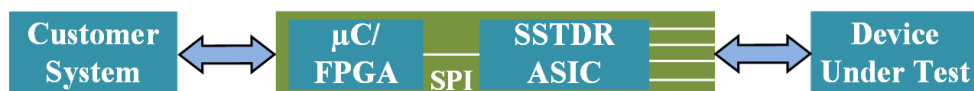
Figure 3.10 A simplified block diagram of the SSTDR-ASIC integration pathway, coined as “Livewire IC” [120].
