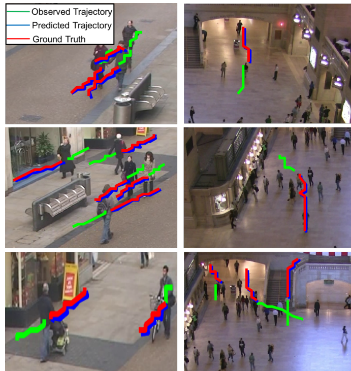
Figure 3.11: Qualitative examples of our method predicting future 12 time steps trajectories, given previous 8 time steps ones on Town Centre (1st column) and Grand Central Station (2nd column) dataset. Note that, we crop and resize the original image for better visualization.
