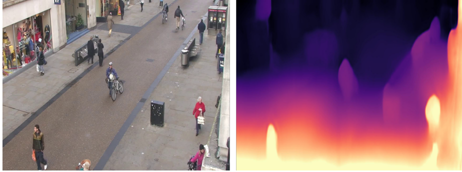
Figure 3.5: Examples of the input (left column) and the output (right column) of the monocular depth estimation [3]. The input image is from Town Centre dataset [4].
