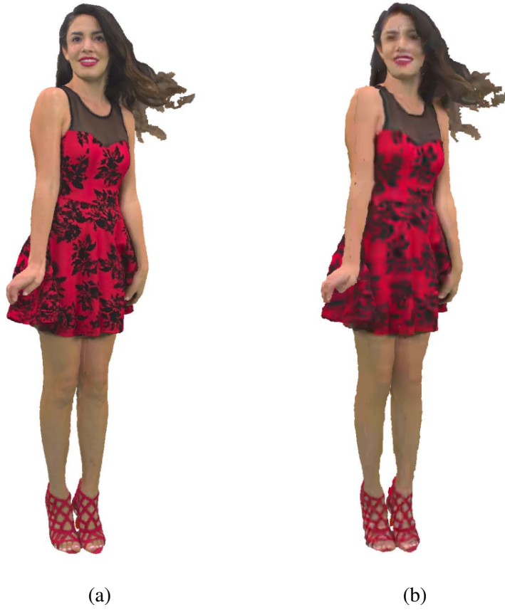
Figure 12: (a) Original (uncompressed) point cloud, (b) Reconstructed point cloud suffering from quantization noise.
