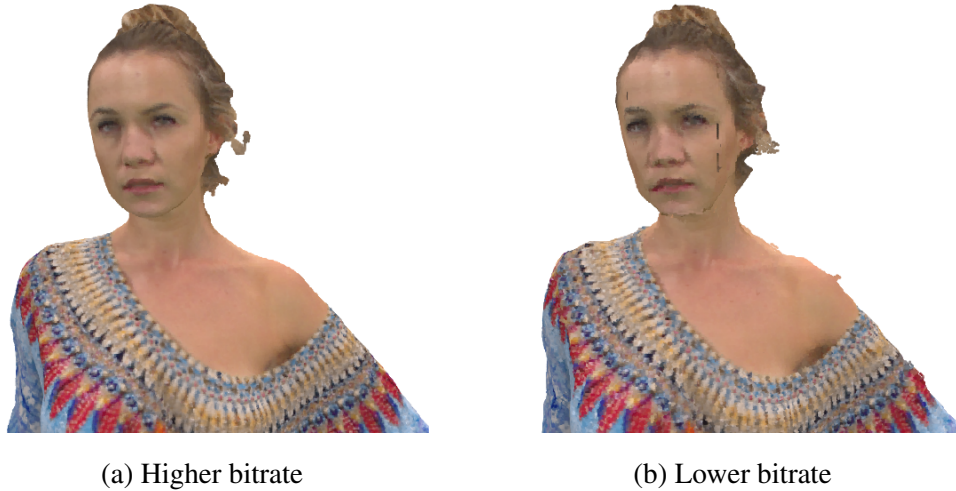
Figure 1: Blocking effects in a point cloud coded at different bitrates using V-PCC encoding.
