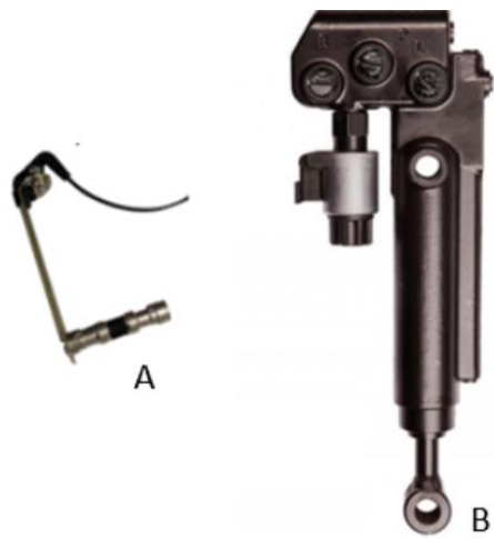
Fig. 3. Precision Planting's load sensing pin (A) and downforce cylinder used with the DeltaForce System.
