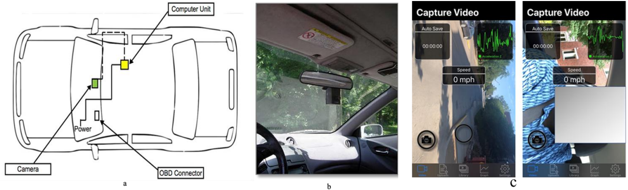
Figure 3. 1.: a) The Positioning of the Blackbox sensors in the vehicle b) Example of the Blackbox sensor inside a vehicle c) Smartphone Data Collection App Interface
