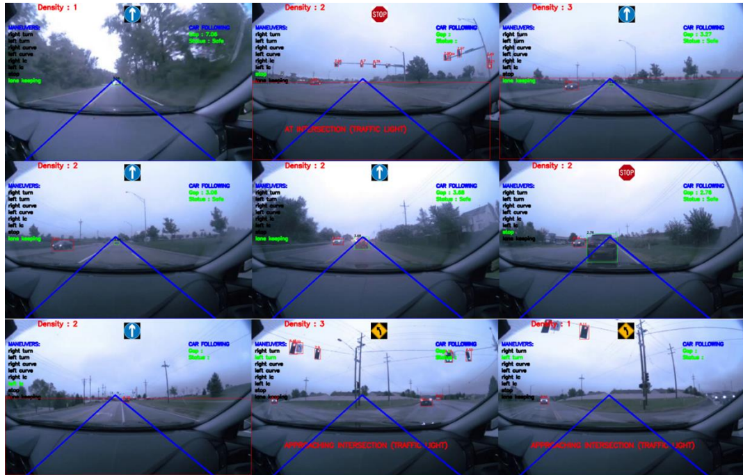
Figure 4. 9: A framework for detecting leading vehicles, safe car-following distance and driver maneuvers.
