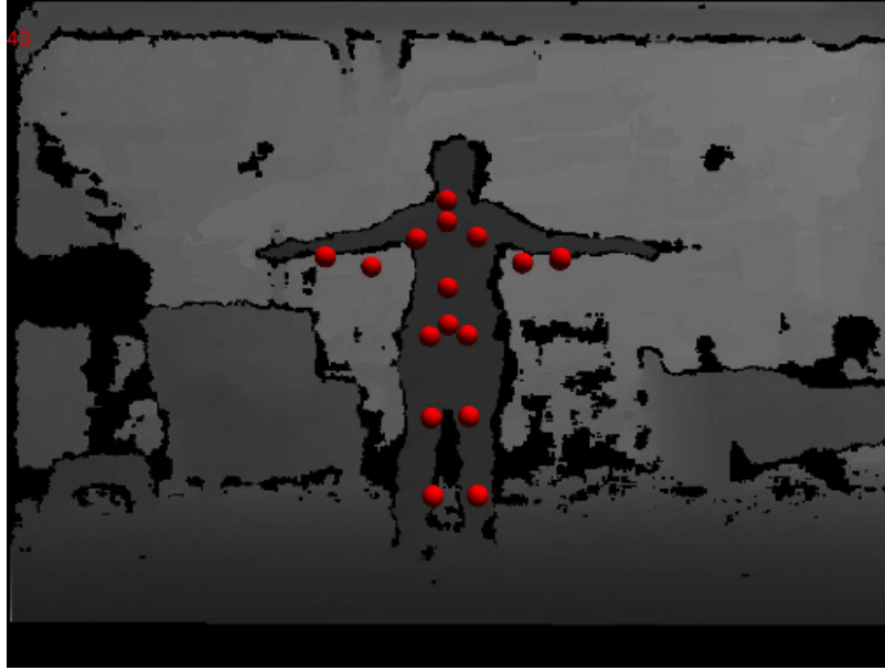
Figure 15. A depth frame and the corresponding skeletal joint data collected from the TVico sensor.
