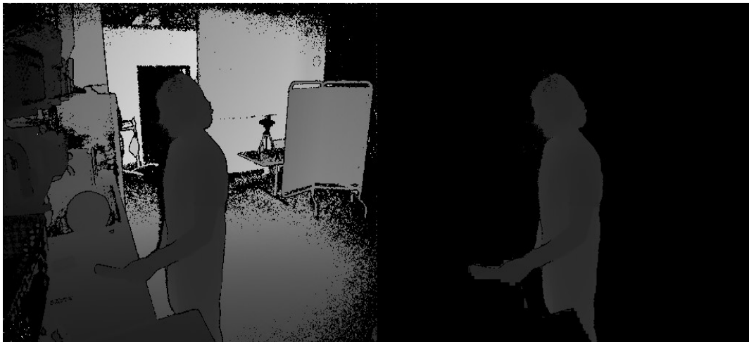
Figure 12. Unprocessed (left) and processed (right) depth data of a subject cutting with a knife.
