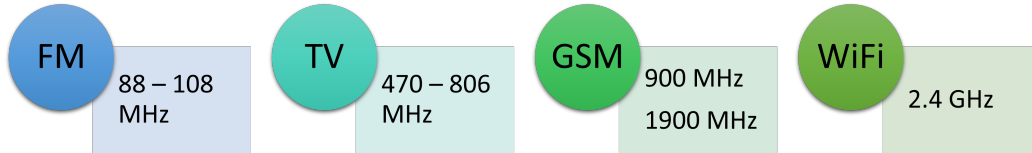
Figure 2.7: Frequency of RF sources [15].
