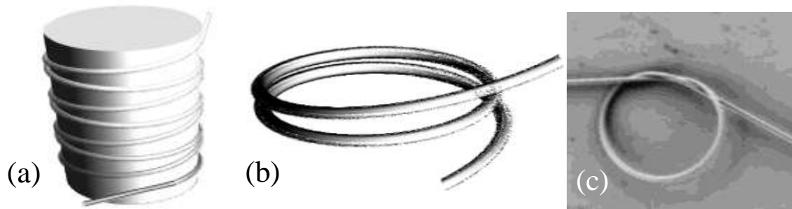
Figure 1.15. A coiled multi-loop resonator (a), double loop microfiber resonator (b), and microknot resonator (c). Reprinted with permission from Tong et al. (2003); Sumetsky (2004).
