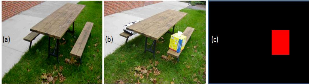
Figure 4.1: 3-D change detection; (a) and (b): two videos taken by different cameras at different times; (c) detection result. The red box represents changes that indicate new object(s).
