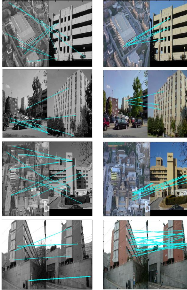
Figure 3.7: building matching performance comparison. Left: results by SIFT-based matching; right: results by this work.
