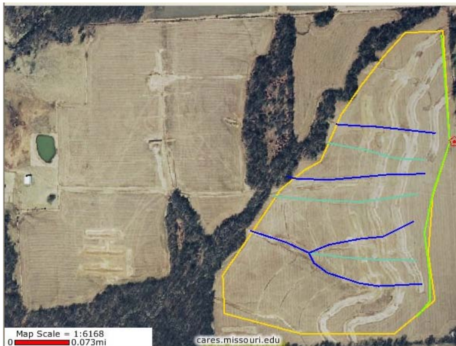
Figure L2.MO599—Pike County Field. Field boundary (yellow), ridgeline(green), outlets(blue), divides(cyan), high point (red point).
