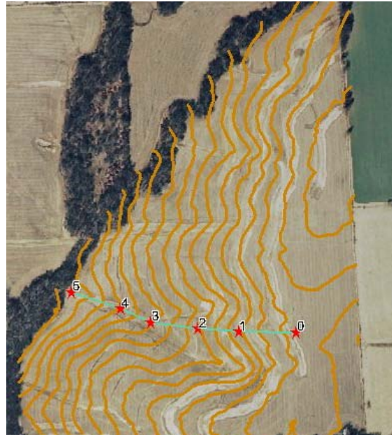
Figure 4.4. Web-Interface view of the divide (cyan) to fall between split streams. Contour line data is shown in orange ( http://www.soilsurvey.org/tools/terrace/main.asp ).
