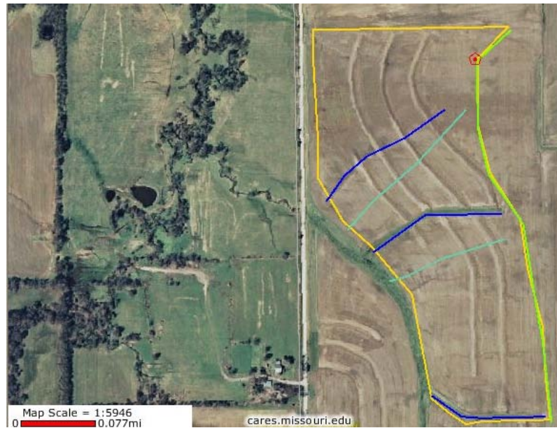
Figure L3.MO574—Monroe County Field. Field boundary (yellow), ridgeline(green), outlets(blue), divides(cyan), high point (red point).
