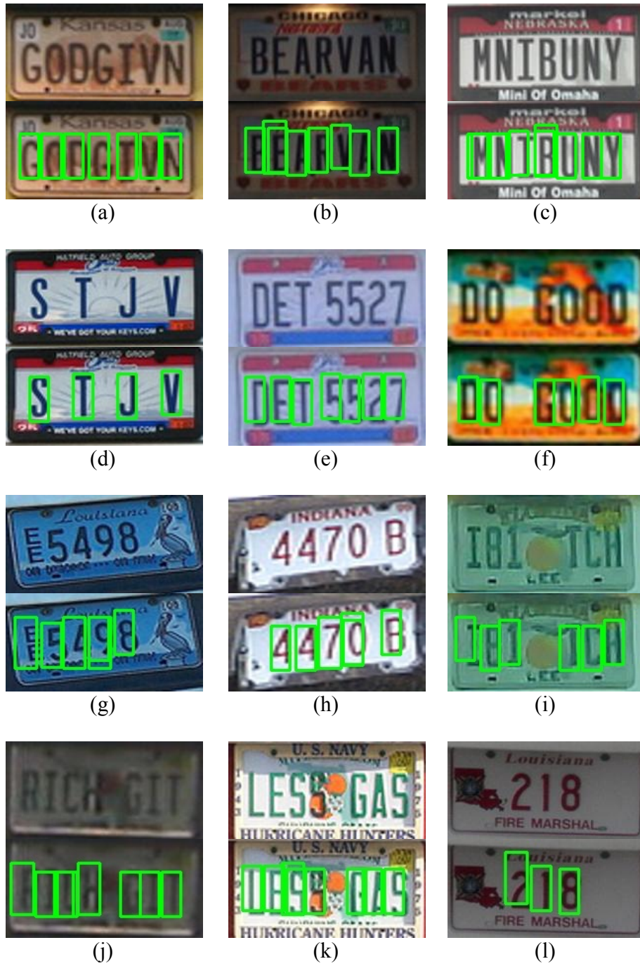
Fig. 3. 1 Character segments of license plates. The original license plates are shown on top of each character segments images. The character segments are labeled by the green bounding boxes.
