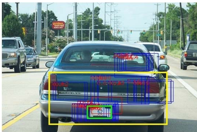
Fig. 2. 6 Fast license plate detection image. The car rear detected is shown in yellow box. License plates are searched within the car rear region. The final license plate detection (shown in green box) is picked out among the potential detections (shown in blue boxes) that merged to the one location (shown in red) by Mean Shift algorithm. The prediction score for each potential prediction is printed in red.
