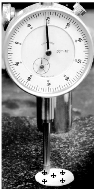
Figure 2.10: Image of a drop pin gauge. The crosses on the sample represent the location of each measurement.
