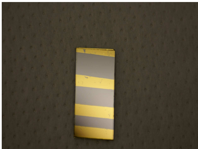
Figure 4.14: Resistance testing using transmission line method.
