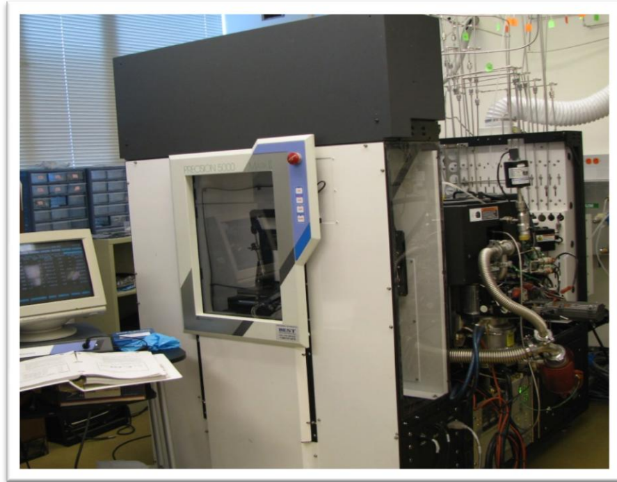
Figure 2-3 Precision 5000 mark II Applied Materials P-5000 RIE etch set-up in Dr. Gangopadhyay's lab.
