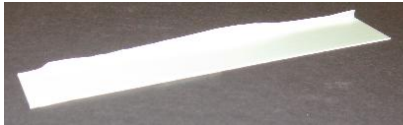
Fig. 4.3. A usable, but unfinished specimen after removal from the original square tube.
