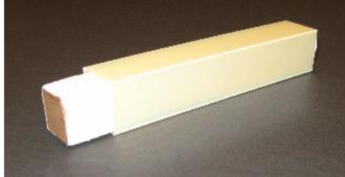
Fig. 4.2. The supportive wooden template used to assist in specimen removal.
