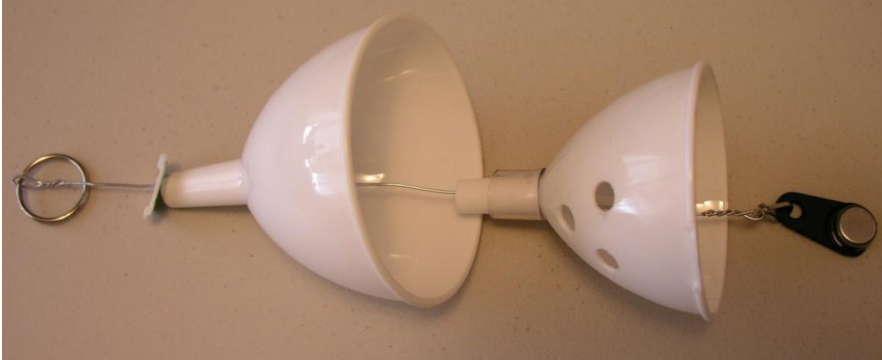
Figure 4: Home built shield used to house iButton temperature and relative humidity sensors from radiation and precipitation, designed by Hubbart (2005). Photo by J.A. Hubbart.
