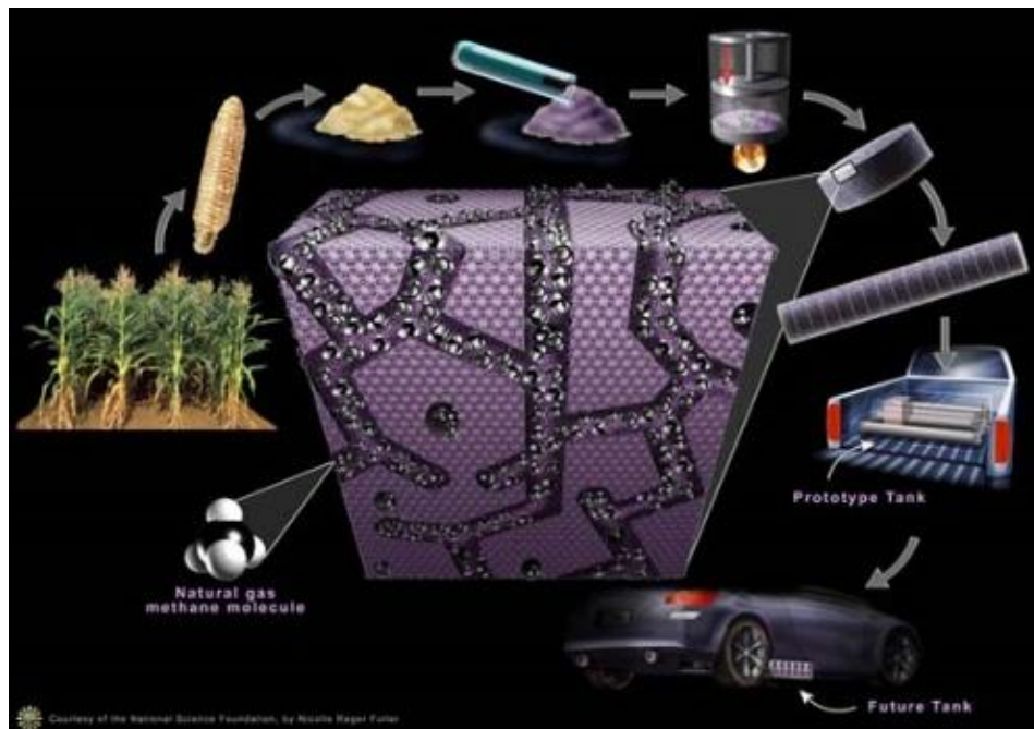
Figure 2. Nanoporous material for vehicular applications—from corn cob to monolith in tank. [18]
