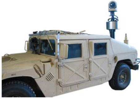
Figure 2.3. US Army NVESD test vehicle showing various mounted cameras.
