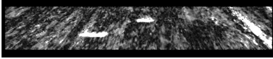
Figure 2.6. Output from the GMM shown as a scaled image. Higher intensity areas correspond to higher confidence that the pixel is foreground. The two bright disks correspond to the targets shown in Figure 2. This image represents a detection window of 640x300 pixels.
