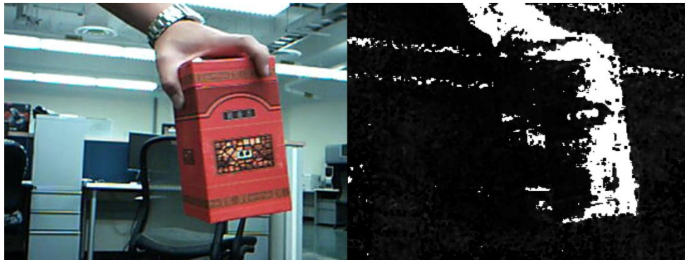
Figure 3.5. GMM run on a simple video of a moving object. In some ways this is more challenging than running on the IR because the box is constantly in frame so the box itself tends to get learned and absorbed into the background if the parameters are not right.
