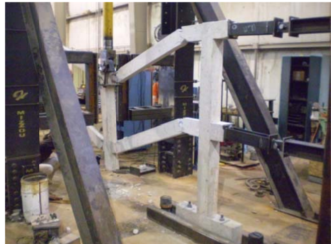
Figure 4.2.4: Continuous frame at failure
