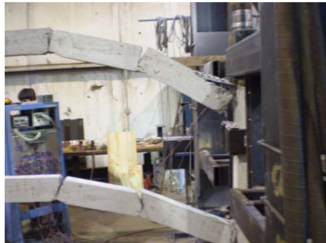
Figure 4.1.3: Discontinuous frame forming hinges
