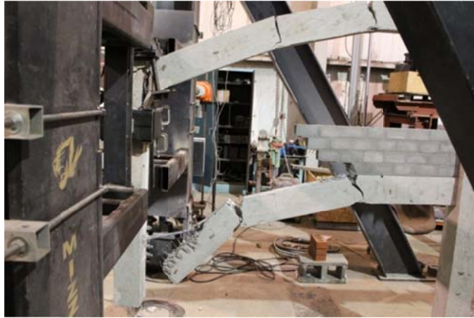
Figure 4.3.14: Negative moment bars have break through stirrups
