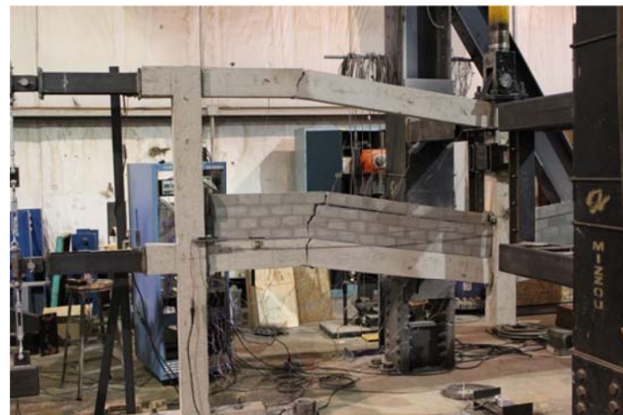
Figure 4.3.6: Infill wall frame forming hinges
