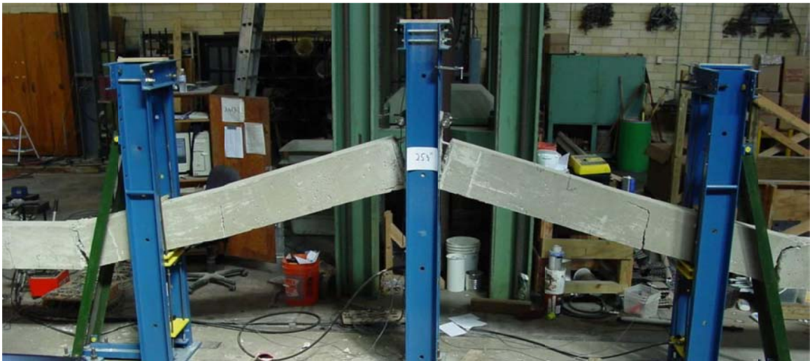
Figure 2.4.5: Photo of test NR-2 under catenary action (Orton, 2007)
