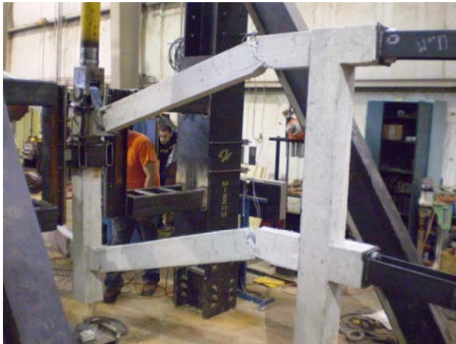
Figure 4.2.3: Continuous frame forming hinges
