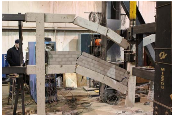
Figure 4.3.8: Infill wall frame at failure
