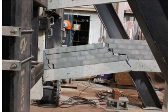
Figure 4.3.11: Crack widens and forms hinge
