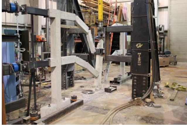
Figure 4.1.4: Discontinuous frame at failure
