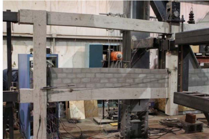
Figure 4.3.4: Infill wall frame forming cracks
