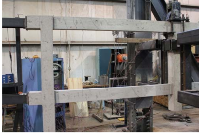
Figure 4.1.1: Discontinuous frame before loading
