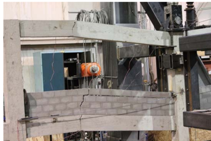
Figure 4.3.5: Infill wall frame cracks widening
