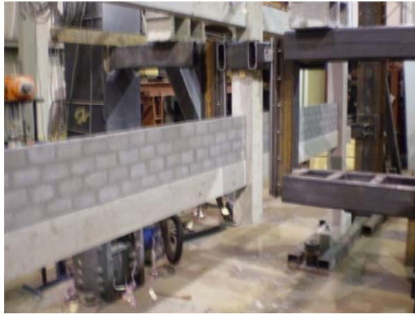
Figure 4.3.1: Side view of infill wall
