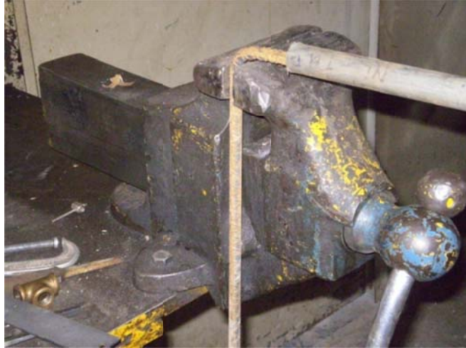
Figure 3.5.8: Bending of longitudinal bar
