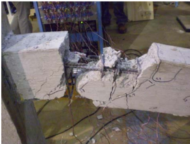
Figure 4.2.8: Concrete falling off
