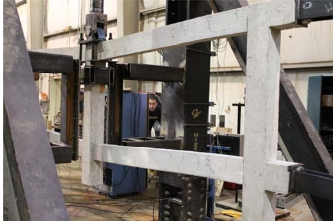
Figure 4.2.2: Continuous frame forming cracks
