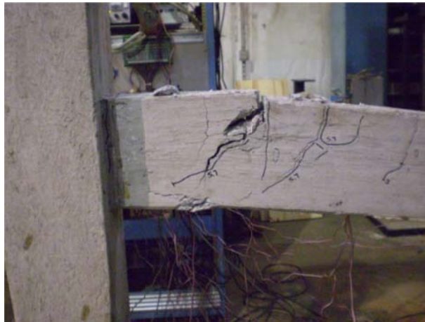
Figure 4.2.7: Formation of hinge
