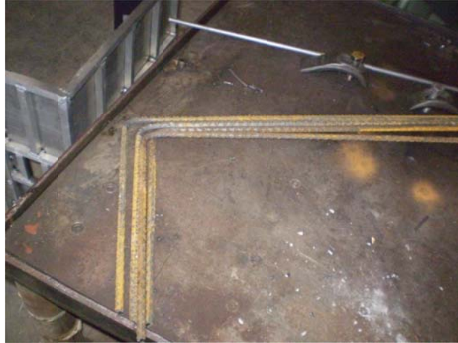
Figure 3.5.11: Bent longitudinal bars
