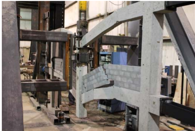
Figure 4.3.12: Infill wall is separated from beam
