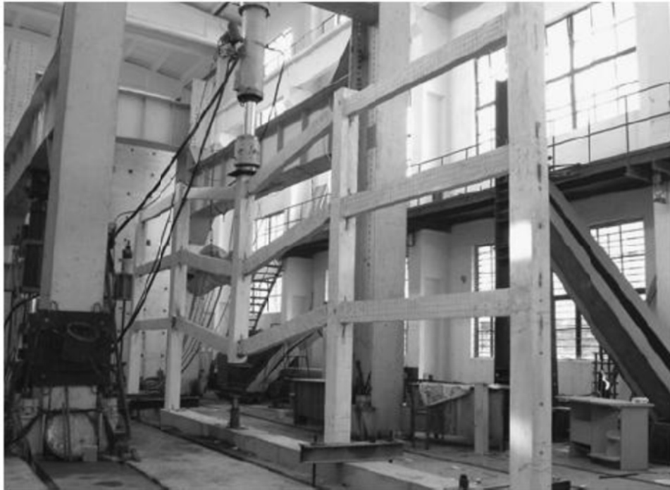
Figure 2.4.7: A reinforced concrete four-bay by three-story one-third scale model frame (Yi and Kunnath, 2008)
