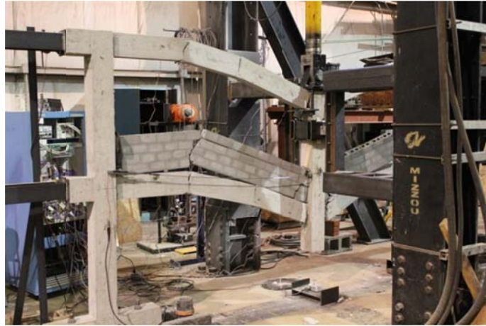
Figure 4.3.7: Infill wall separating from beam
