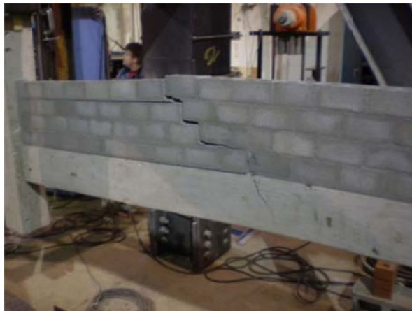
Figure 4.3.9: Crack forms in infill wall
