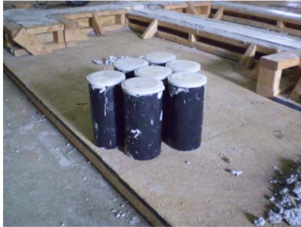
Figure 3.5.23: Compression test cylinders
