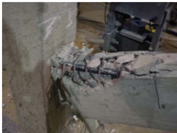
Figure 4.1.9: Formation of hinges at the center column
