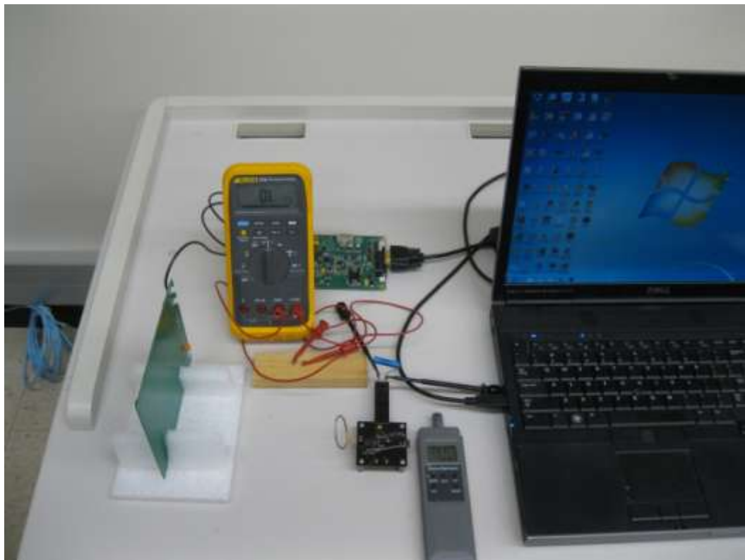
Figure 5.10 Measuring resistance of wood with Fluke 87 DMM
