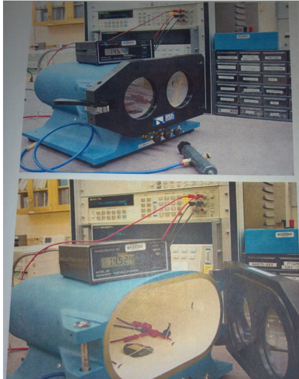
Figure 3.1: (Top) The MEMS sensor in a closed pressure chamber being read by an Agilent 3458 DMM. (bottom) Pressure chamber opened to expose the MEMS sensor
