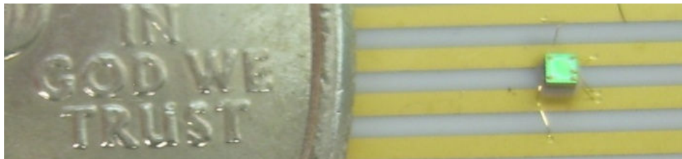
Figure 2.2: Wire bonded pressure sensor next to U.S. dime.
