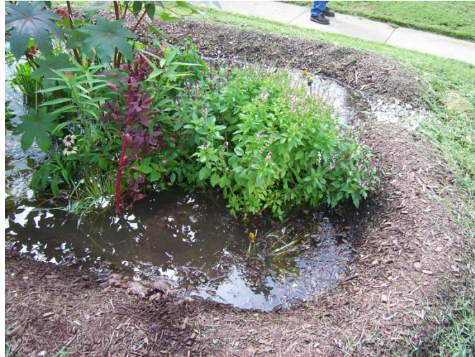
Figure 6.3 Water pool during full-inundation infiltration test.
