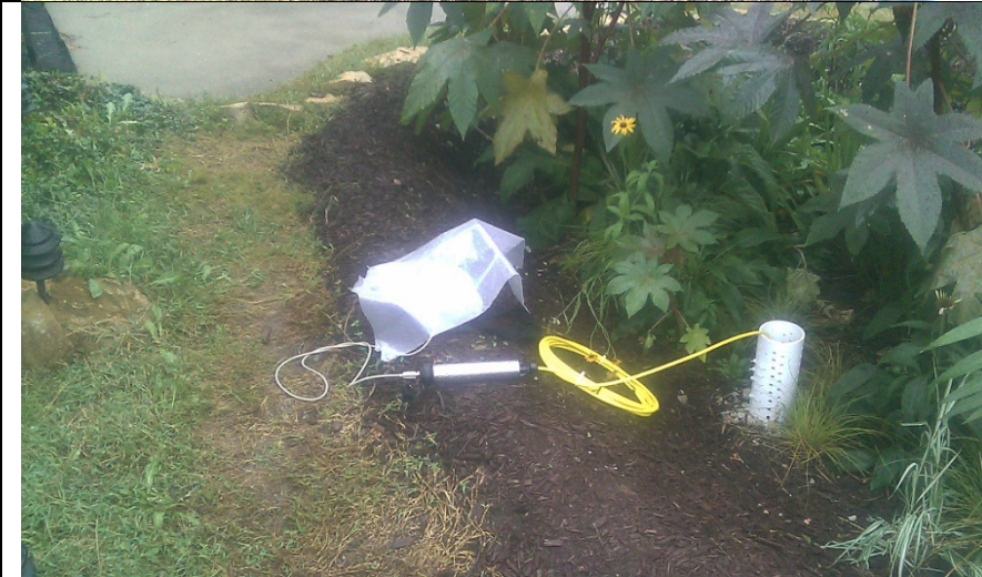
Figure 3. Data collection from rain garden Global Water Level Logger WL16. 10/11/10
