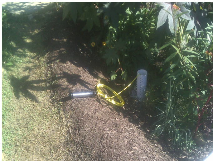
Figure 7.2 Level logger in rain garden absorption area.
