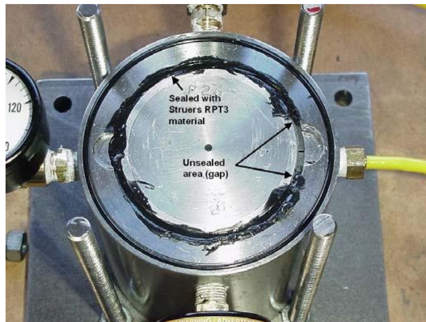
Figure 9: Piston cylinder interface sealed with cylinder head gasket sealant [17].
