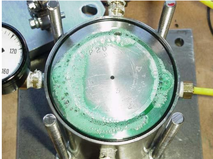
Figure 8: Gas, oil, and soap bubbling from the top of the piston at the piston/cylinder interface [17].
