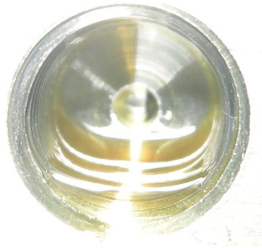
Figure 43 Real valve opening geometry
