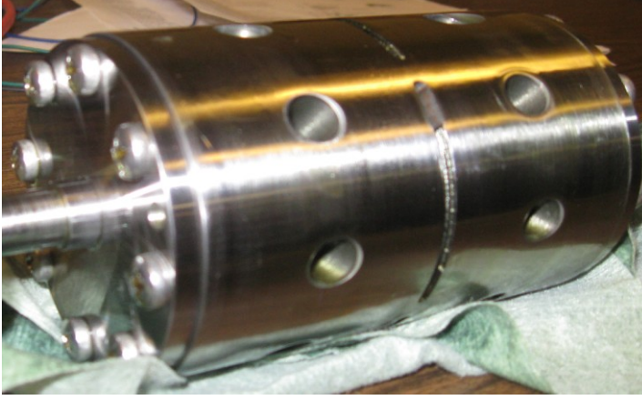
Figure 18 Modified rotor and pass-partition plate design
