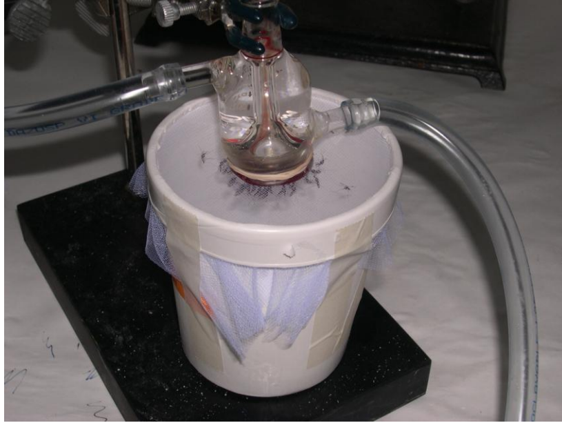
Figure 2.1. Membrane feeding apparatus used for infecting Anopheles stephensi with Plasmodium falciparum . Mixed gametocyte cultures that had been induced for 16 days were fed to An. stephensi for 30 minutes using a water-jacketed membrane feeding system set to 37°C.
