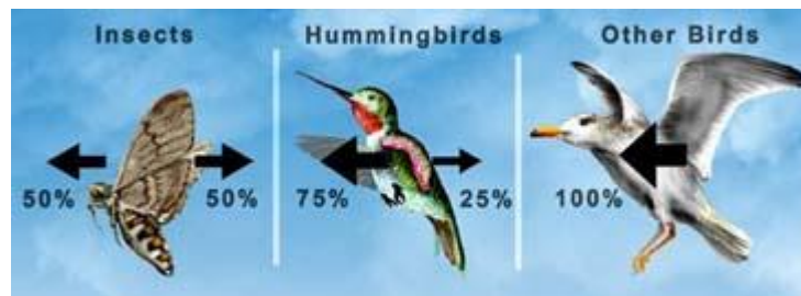
Fig. 2-42. Lift production on downstroke vs. upstroke in insects, hummingbirds, and birds.
