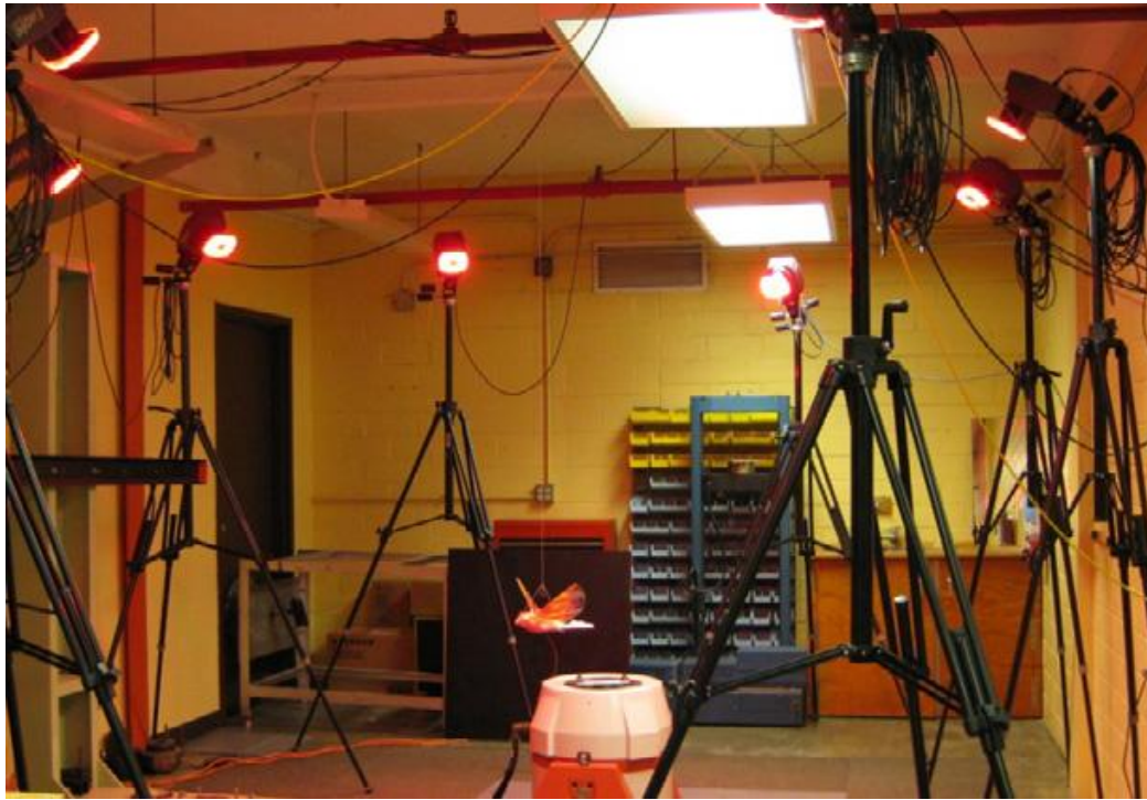
Fig. 5-2. EAGLE-500 camera-based motion analysis system.
