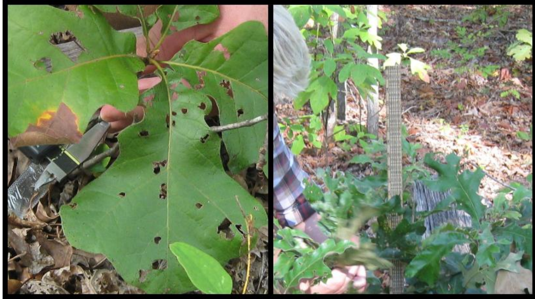
Figure 6. Left: Digital calipers used to measure basal diameter. Right: Biltmore stick used to measure height of understory trees.
