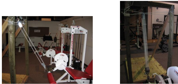
Figure 2. Compound pulley system for the leg extension was anchored to a support frame, constructed by researchers, and the class 2 pulley was attached to the lever arm of the leg extension by a U-bolt attached to an eye bolt. Pulley system was used to raise weight for ECC and lower weight for CON group.
