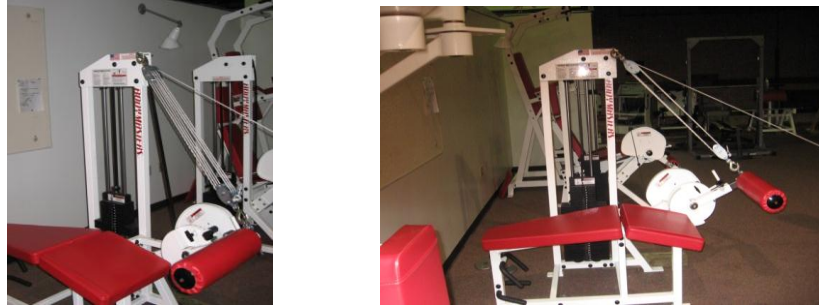
Figure 1. Pulley set-up for CON and ECC group. Attachment of compound pulley system to the leg curl machine. Pulley system was anchored to the top of the weight tower. Pulley system was used to assist researchers in lifting weight for ECC and lowering weight for CON group.
