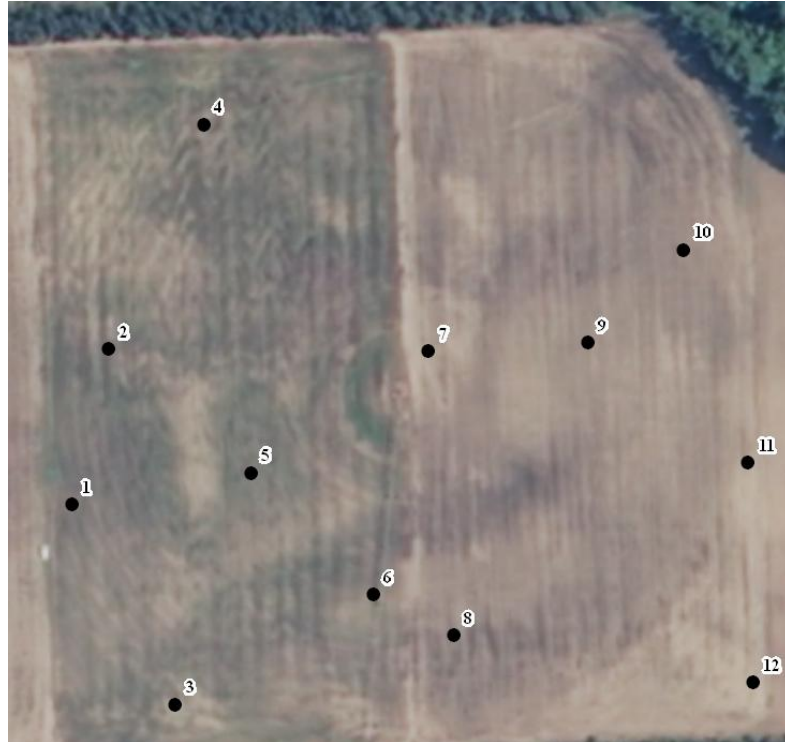
Figure 4.3: Location of soil sample cores collected for calibration of Veris EC a data (2002).
