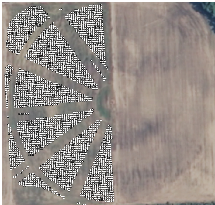
Figure 3.17: Yield data from 2010 kriged to a 3-m grid corresponding with sand content data from 2002.
