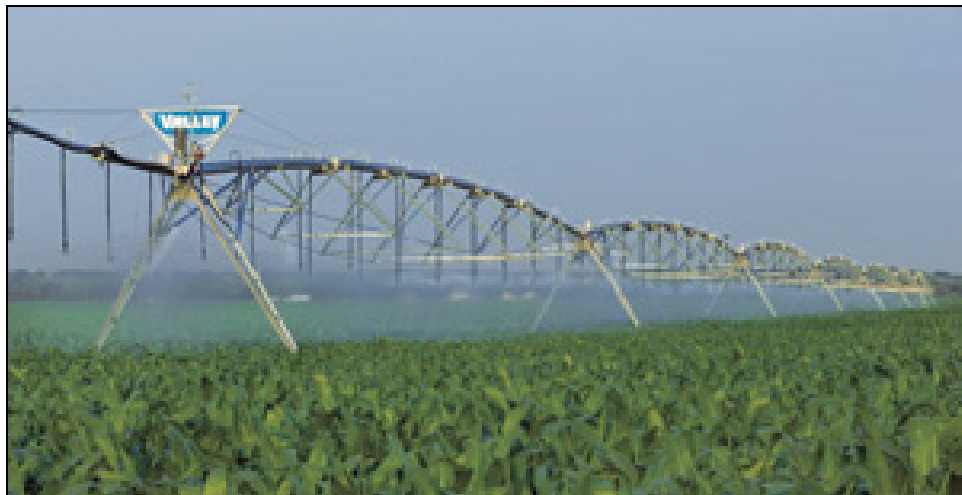
Figure 1.2: 8000 series center-pivot by Valley Manufacturing ( www.valleyirrigation.com )
