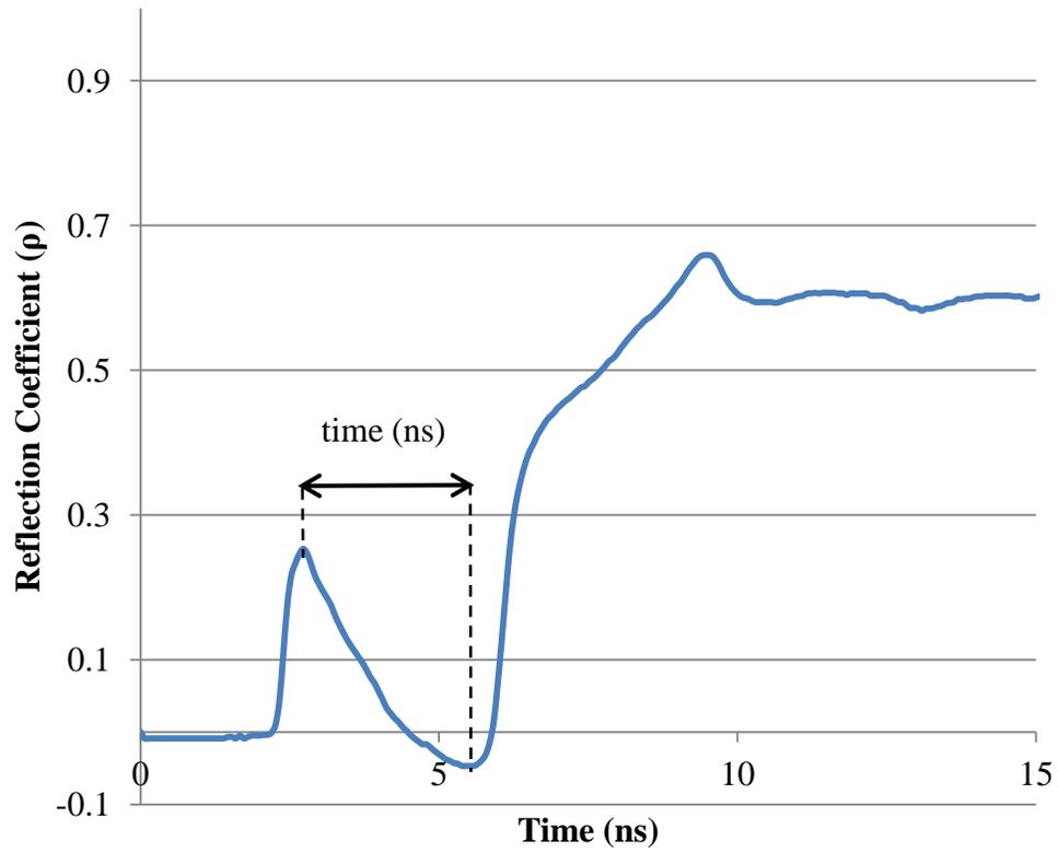
Figure 3-7. Procedure for determination of “time” for dielectric constant calculation.
