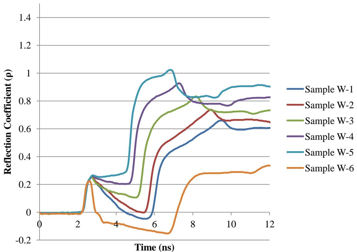
Figure 4-1. TDR waveforms for Wet Condition.
