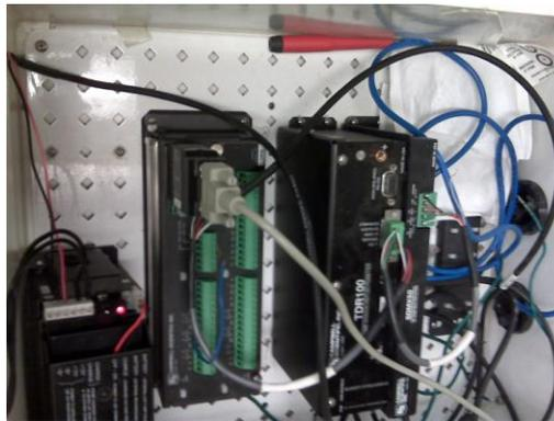
Figure 3-1. TDR pulse generator and multiplexer
