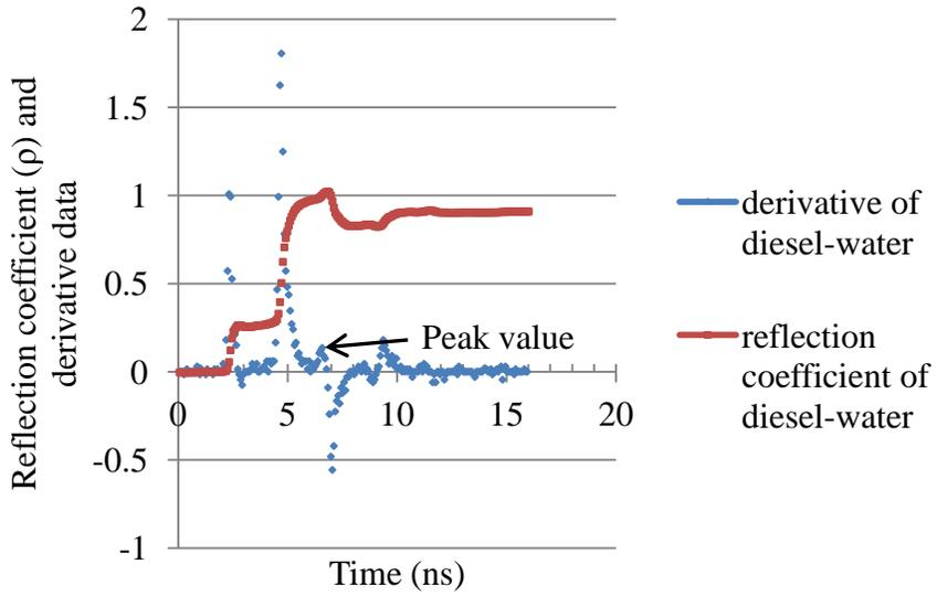
Figure 4-5. TDR waveform and derivative data for Sample no. W-1
