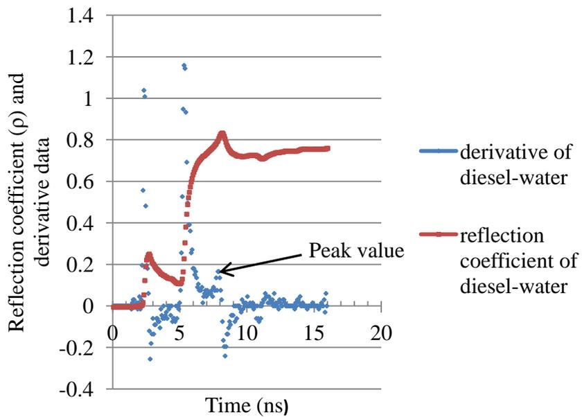
Figure 4-8. TDR waveform and derivative data for Sample no. W-4
