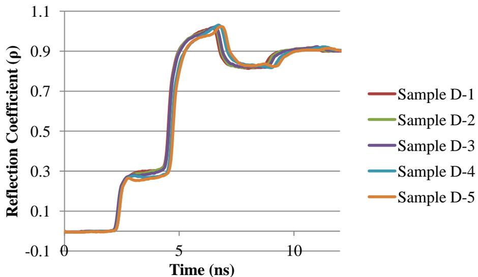
Figure 4-2. TDR waveforms for the Dry Condition
