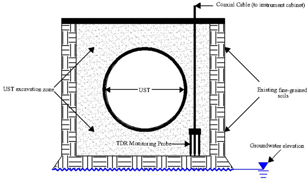
Figure 3-6. Dry Condition (not to scale).
