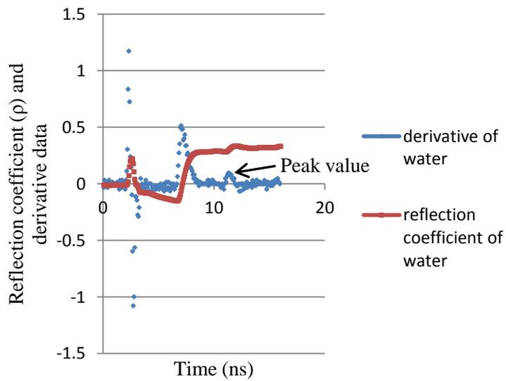
Figure 4-12. TDR waveform and derivative data for Sample no. N-3
