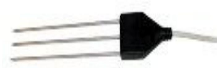
Figure 3-2. TDR monitoring probe
