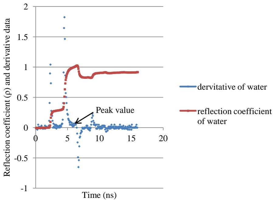
Figure 4-10. TDR waveform and derivative data for Sample no. N-1
