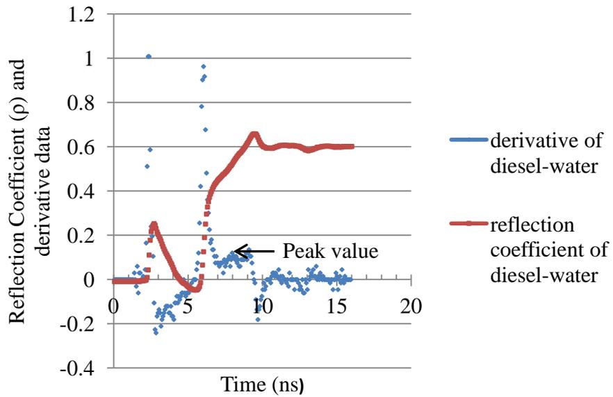
Figure 4-6. TDR waveform and derivative data for Sample no. W-2
