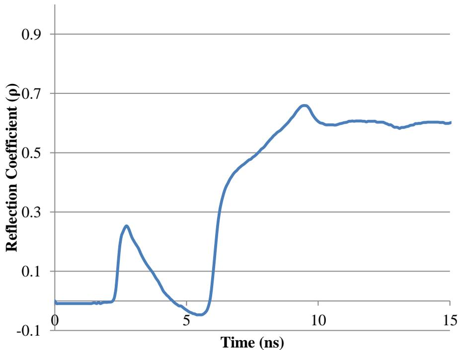
Figure 3-3. Sample TDR waveform from PC-TDR software.
