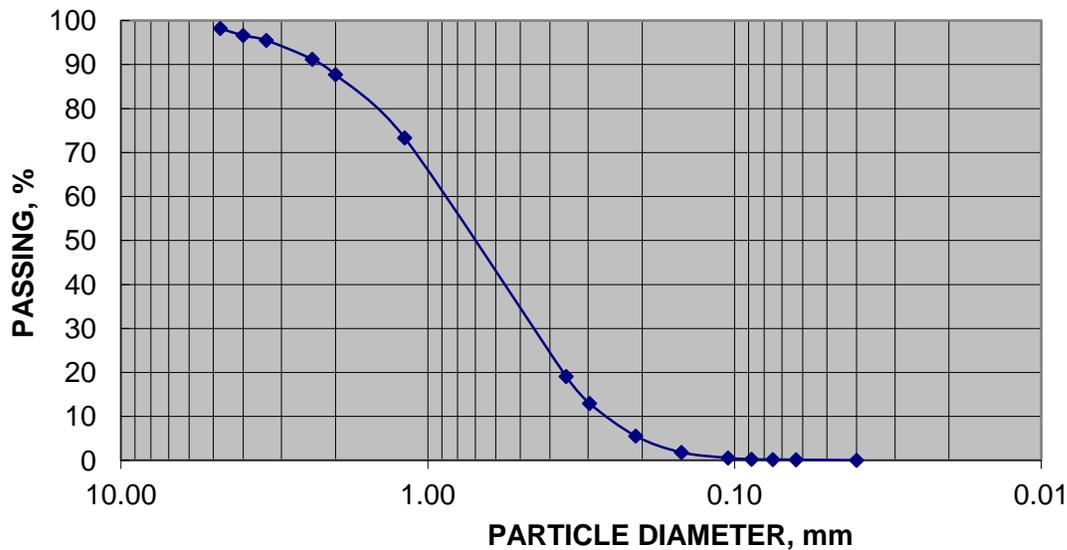
Figure 3-4. Grain size distribution curve for tested samples.
