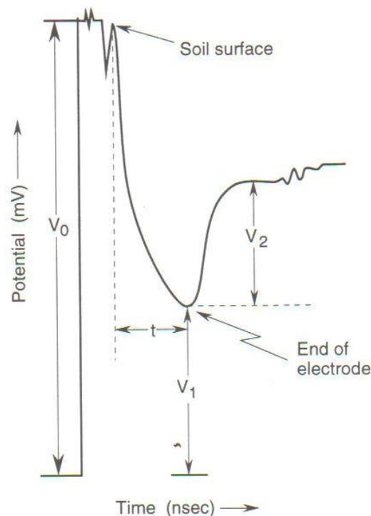
Figure 1-1. Typical TDR waveform (O'Connor and Dowding, 1995).
