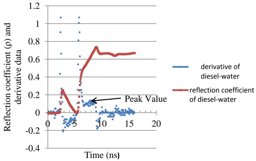
Figure 4-7. TDR waveform and derivative data for Sample no. W-3
