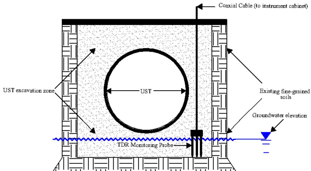
Figure 3-5. Wet Condition (not to scale).
