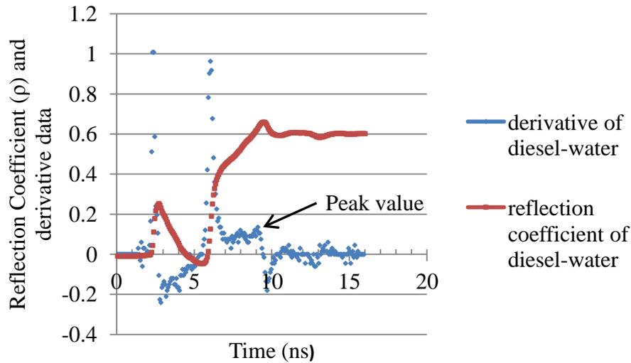
Figure 4-9. TDR waveform and derivative data for Sample no. W-5
