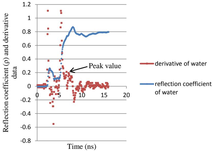
Figure 4-11. TDR waveform and derivative data for Sample no. N-2
