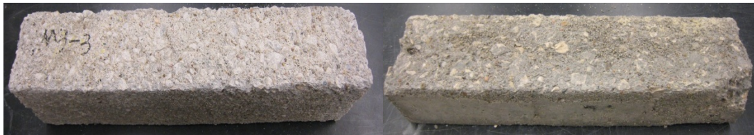
Figure.33 PLC10 (10% limestone) on the left, PLC15 (15% limestone) on the right
