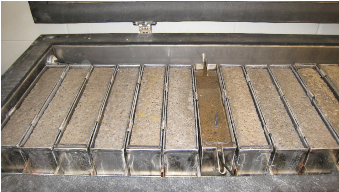
Figure.7 Saturated Freeze-Thaw Samples in the Tank
