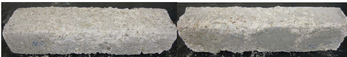
Figure.36 PL15F5 (15% limestone, 5% fly ash) on the left, PL18F2 (18% limestone, 2% fly ash) on the right
