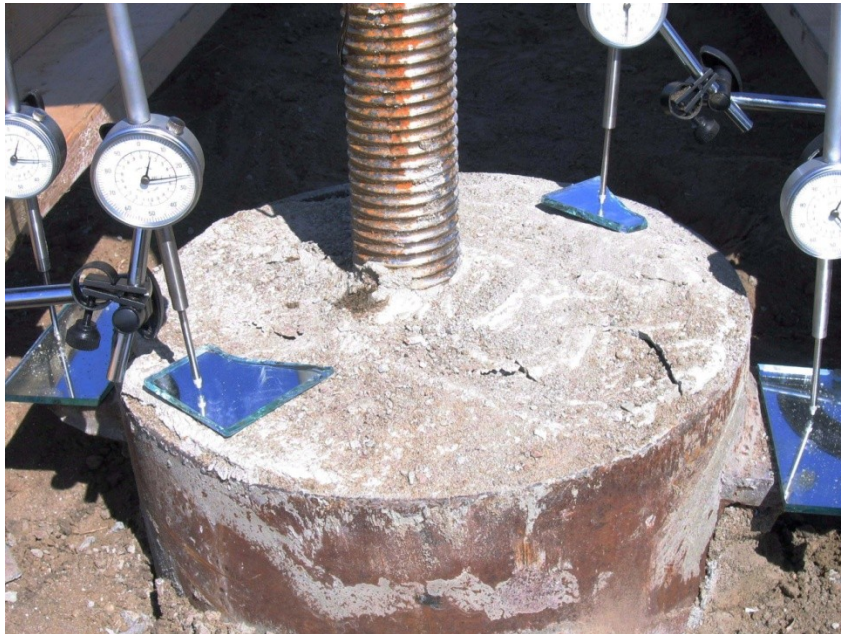
Figure 9: Dial gauges for monitoring pile top movement.
