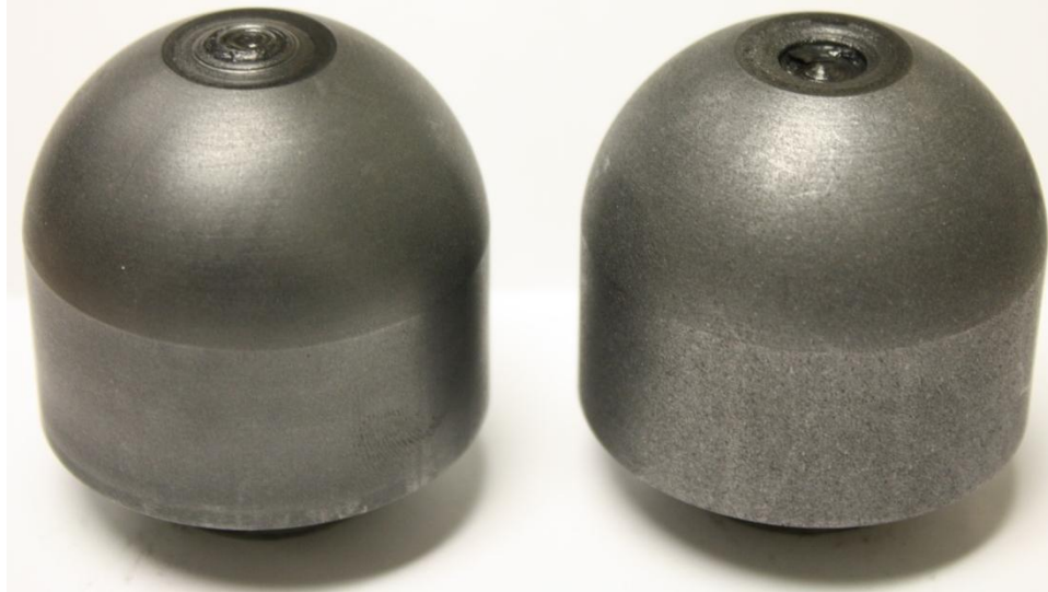
Fig. 7. Samples of 56 kg test exhibiting concave/convex shape. Rotated sample on left.
