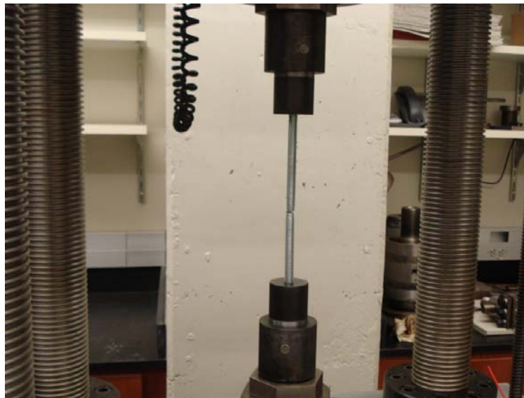
Figure 22: Typical Observed Failure of Tensile Test Specimen
