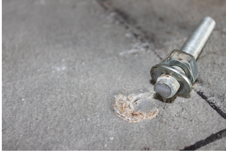
Figure 78: Typical Shear Failure Experienced by Bottom (Rear) Steel Anchor Elements of Test Group B
