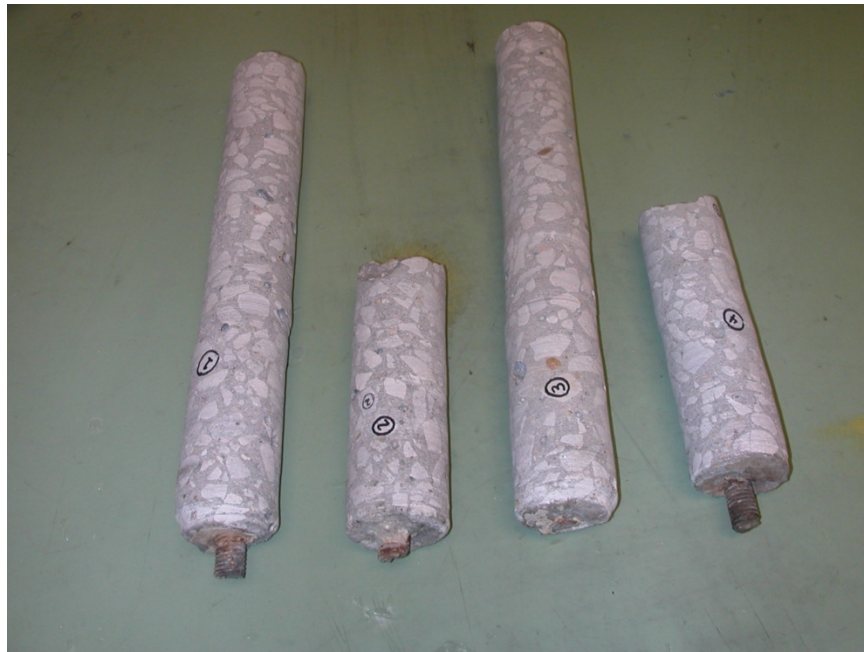
Figure 91: Four Core Samples taken from Test Groups A and B
