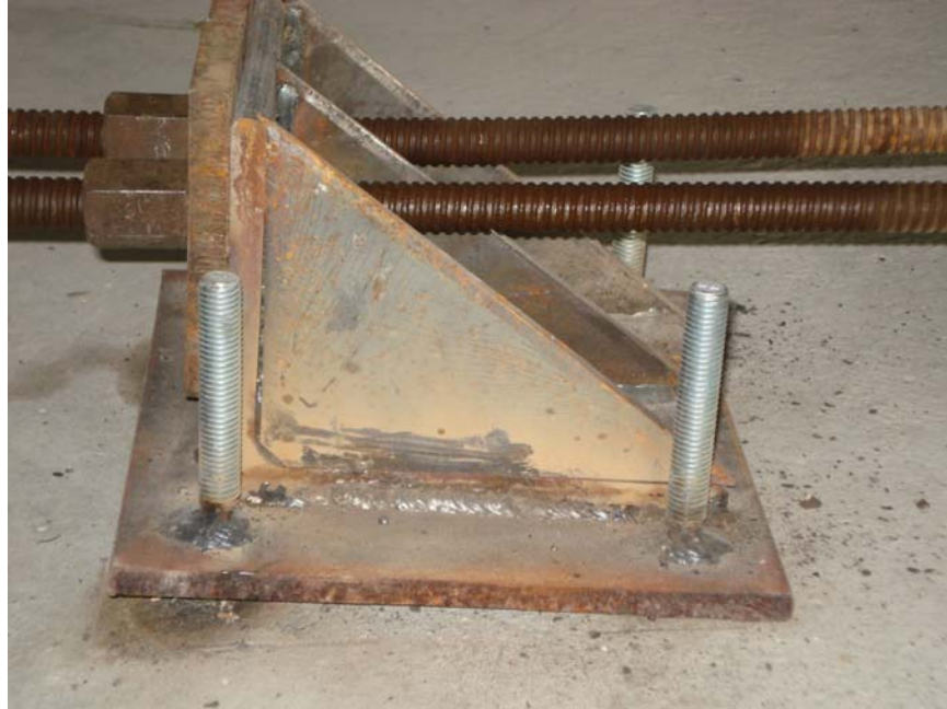
Figure 84: Prying of Corner of Test Group C Test Specimen due to Shear and Tension Failure of Single Top (Load Side) Steel Anchor Element
