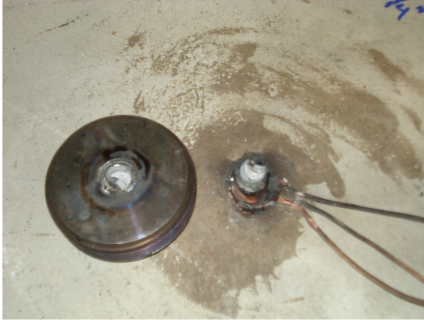
Figure 51: Weld Failure of Test Group L Welded Test
