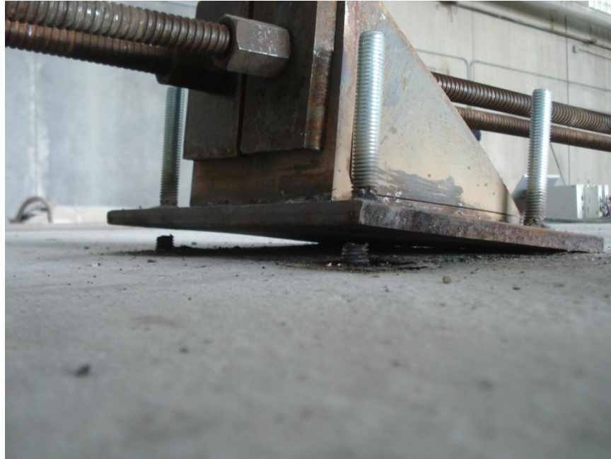
Figure 82: Test Group C Shear and Tension Failure of Two Top (Load Side) Steel Anchor Elements
