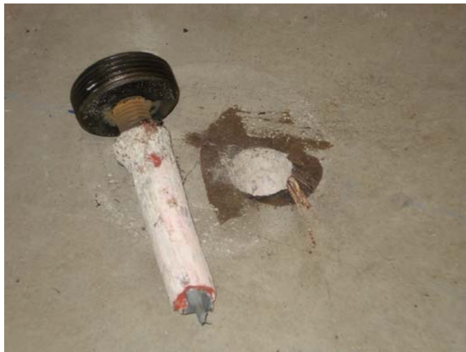
Figure 57: Bond/Borehole Failure of Test Group M Welded Test
