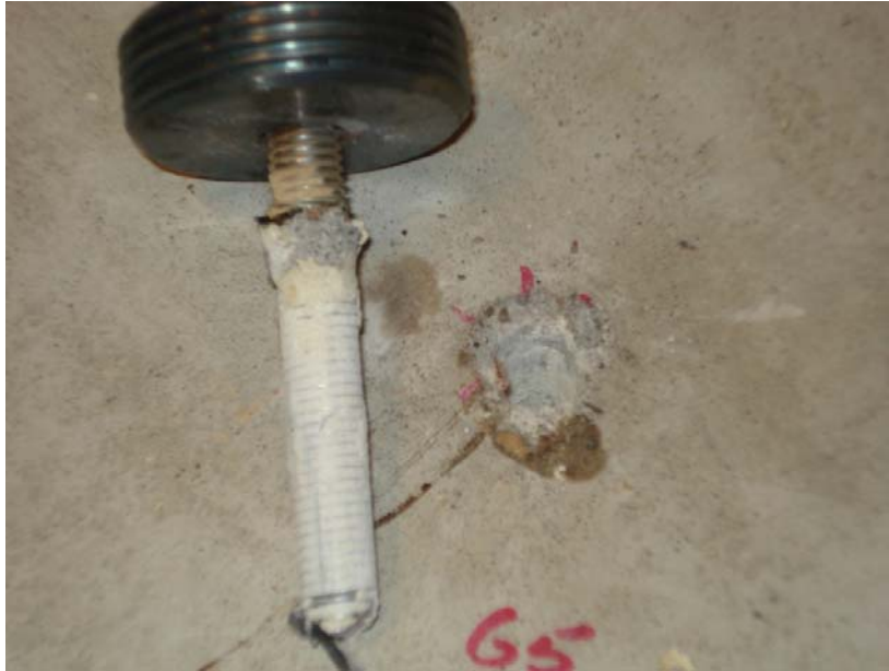
Figure 42: Mixed Bond Failure of Test Group H Welded Test
