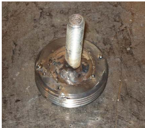
Figure 33: Fillet Welded Test Specimen
