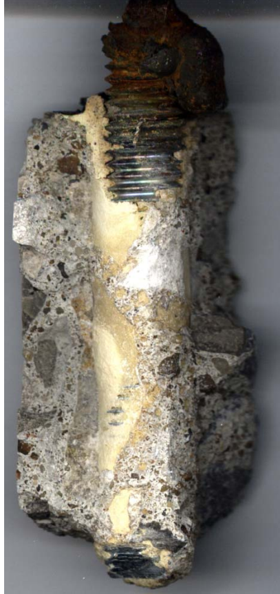
Figure 65: Split Core Sample from Welded Confined Static Tension Test
