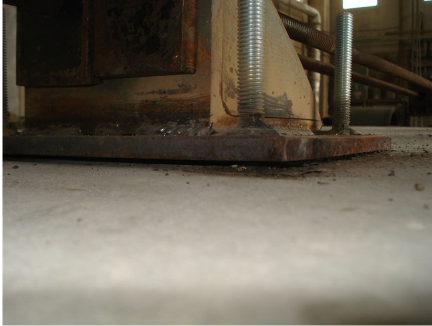
Figure 83: Test Group C Shear and Tension Failure of Single Top (Load Side) Steel Anchor Element
