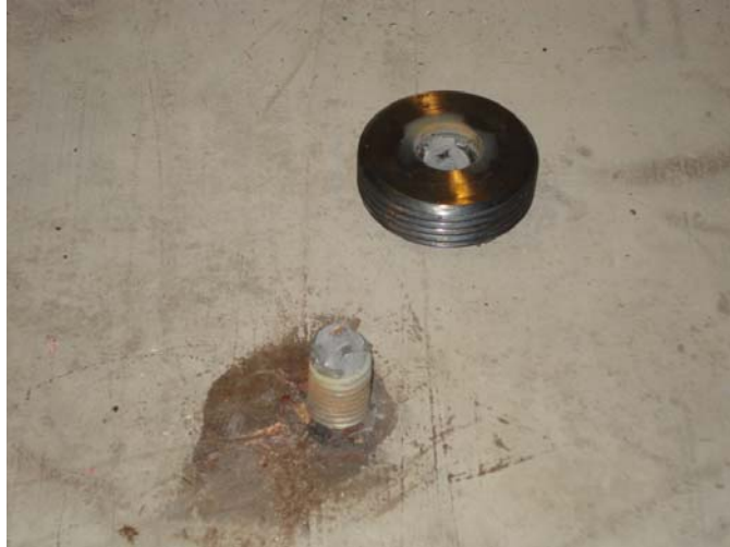
Figure 56: Steel Anchor Element Failure of Test Group M Welded Test
