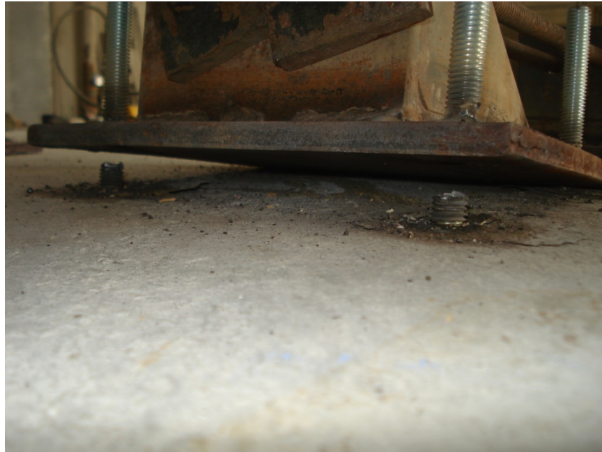
Figure 85: Test Group C Projection of Top (Load Side) Steel Anchor Elements from Concrete Surface
