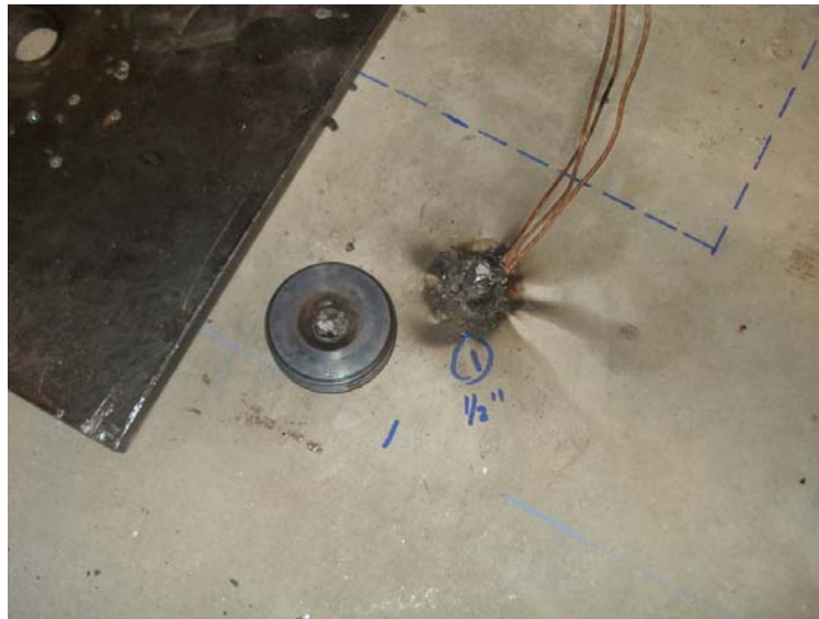
Figure 45: Weld Failure of Test Group J Welded Test
