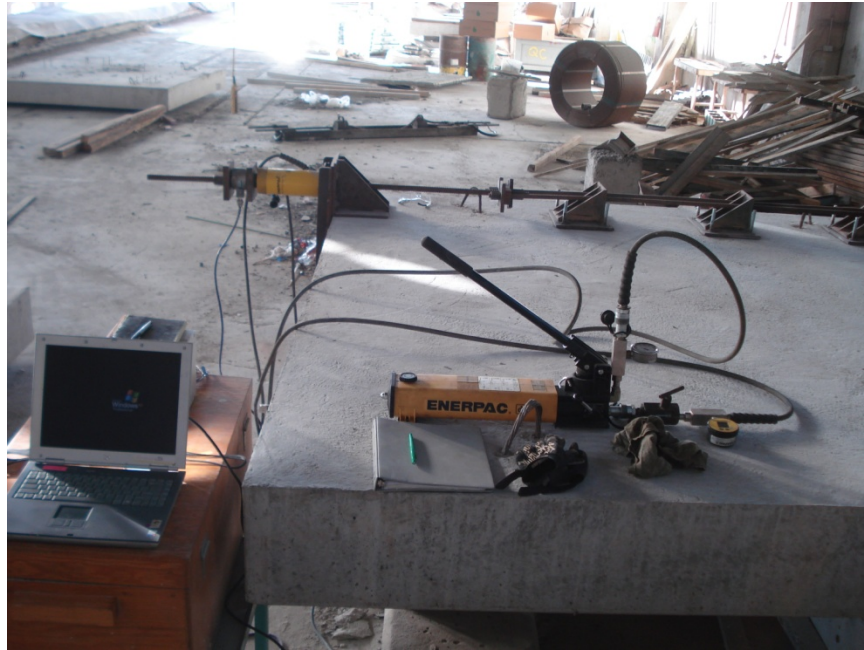
Figure 20: Overall Testing Configuration of Eccentric Shear Tests
