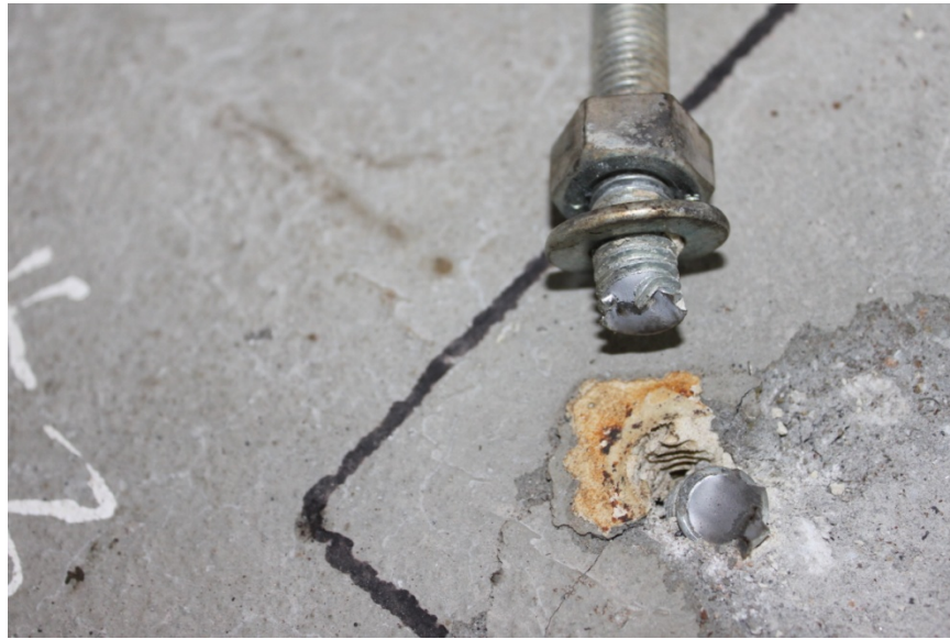
Figure 76: Typical Shear and Tension Failure Experienced by Test Group B Steel Anchor Elements
