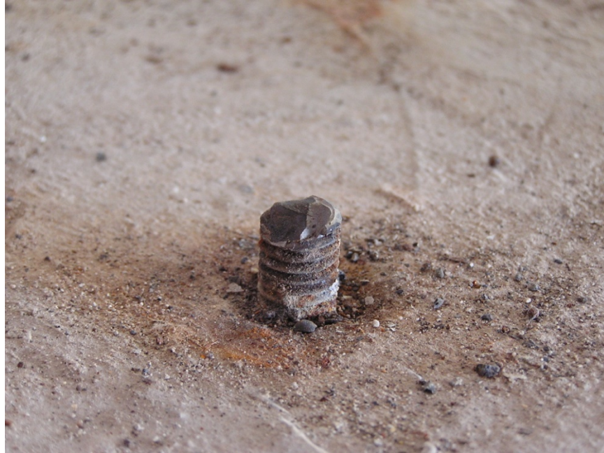
Figure 71: Test Group A Projection of Top (Load Side) Steel Anchor Element from Concrete Surface
