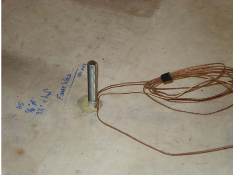
Figure 35: Installed Anchor with Thermocouples
