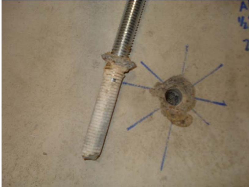
Figure 40: Bond/Element Failure of Test Group H Reference Test
