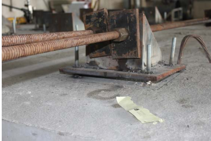
Figure 69: Test Group A Rotational Displacement Due to Weld Failures at Steel Anchor Elements
