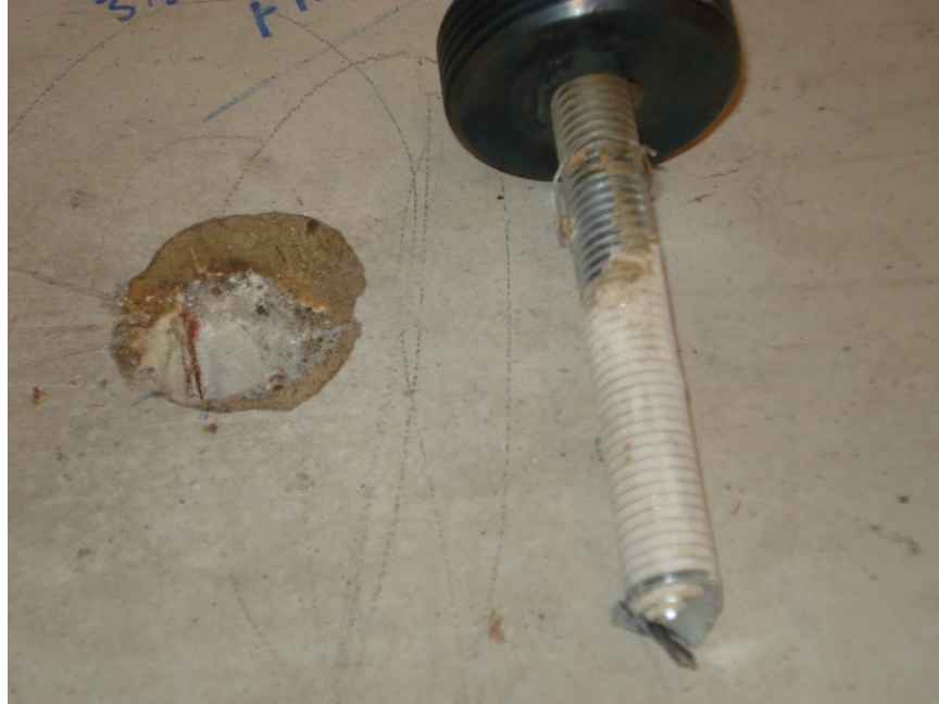
Figure 44: Bond/Element Failure of Test Group I Welded Test
