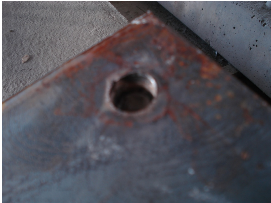
Figure 87: Test Group C Steel Anchor Element Failure Plane near the Root Weld Plane
