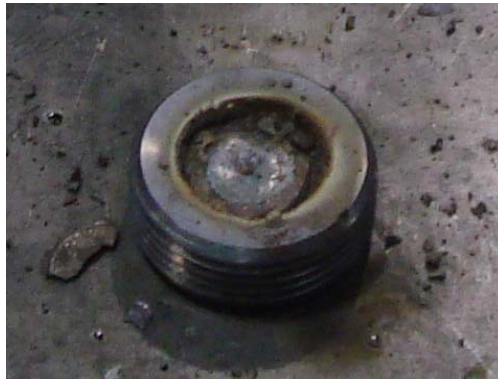
Figure 32: Plug Welded Test Specimen
