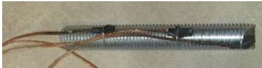
Figure 34: Thermocouple Attachment to HAS Steel Element
