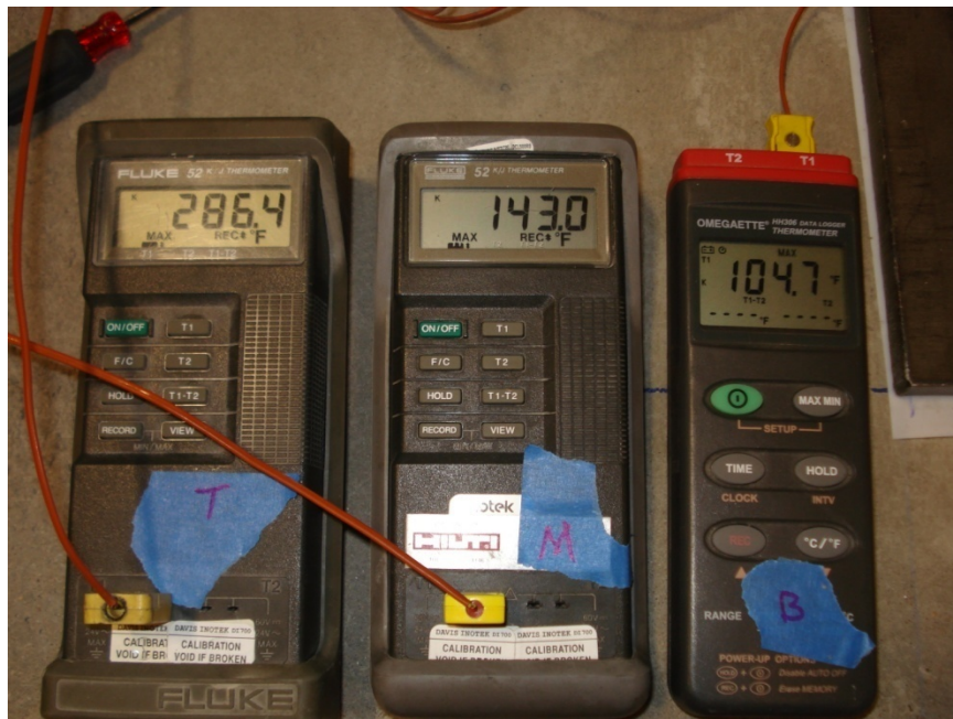
Figure 37: Handheld Thermometers used to Record Temperature during Welding
