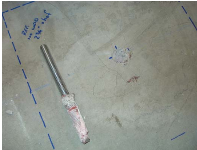
Figure 49: Mixed Bond Failure of Test Group L Reference Test
