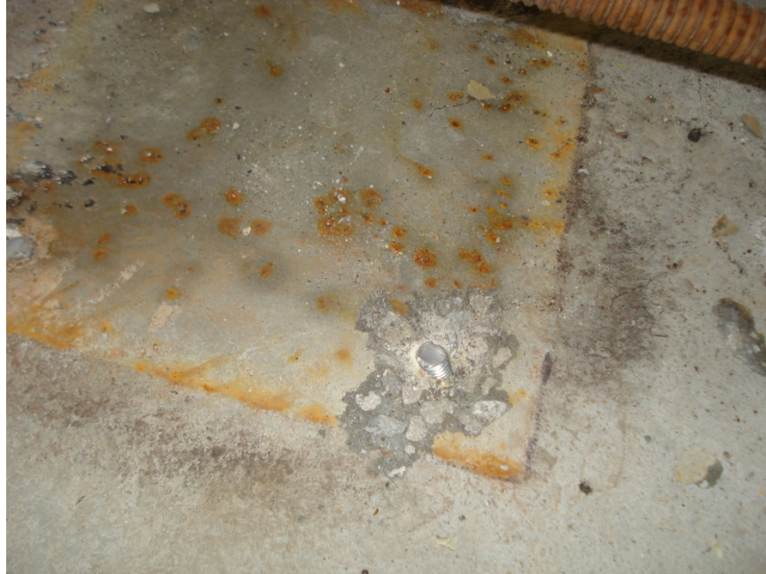
Figure 77: Concrete Cone and Spalling Observed around Top (Load Side) Steel Anchor Elements of Test Group B
