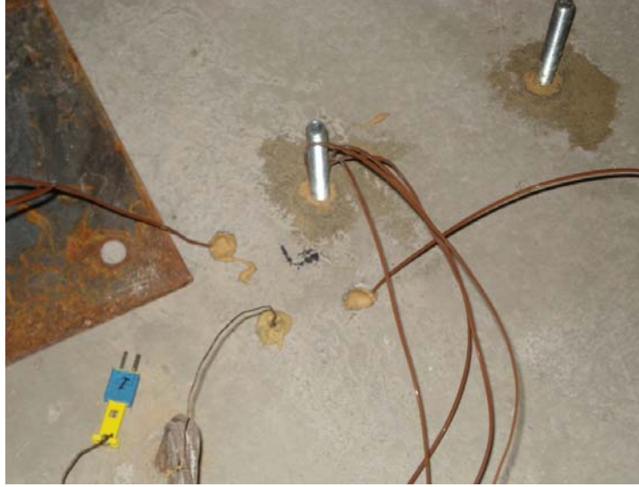
Figure 25: Installed Thermocouples for Single Anchor of Temperature Gradient Test
