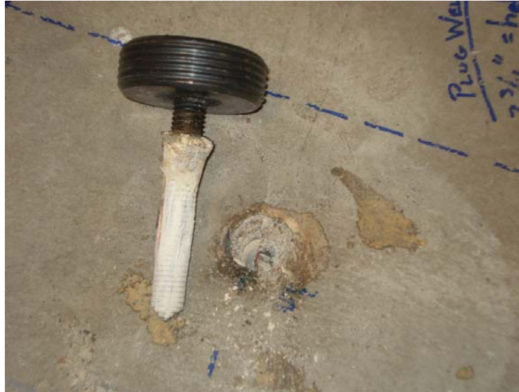
Figure 46: Bond/Element Failure of Test Group J Welded Test
