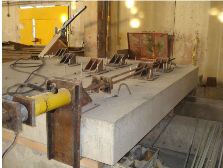
Figure 18: Configuration of High-strength Rods and Hollow Plunger Cylinder
