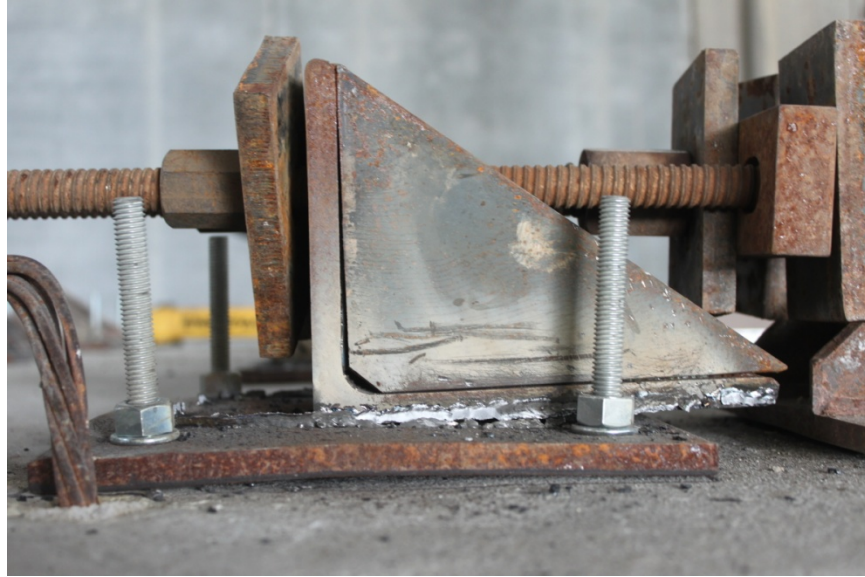
Figure 74: Test Group B Weld Failure between the Stiffened Seat and Base Plate
