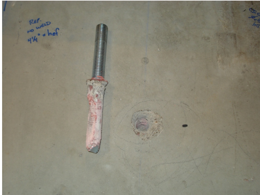
Figure 54: Mixed Bond Failure of Test Group M Reference Test
