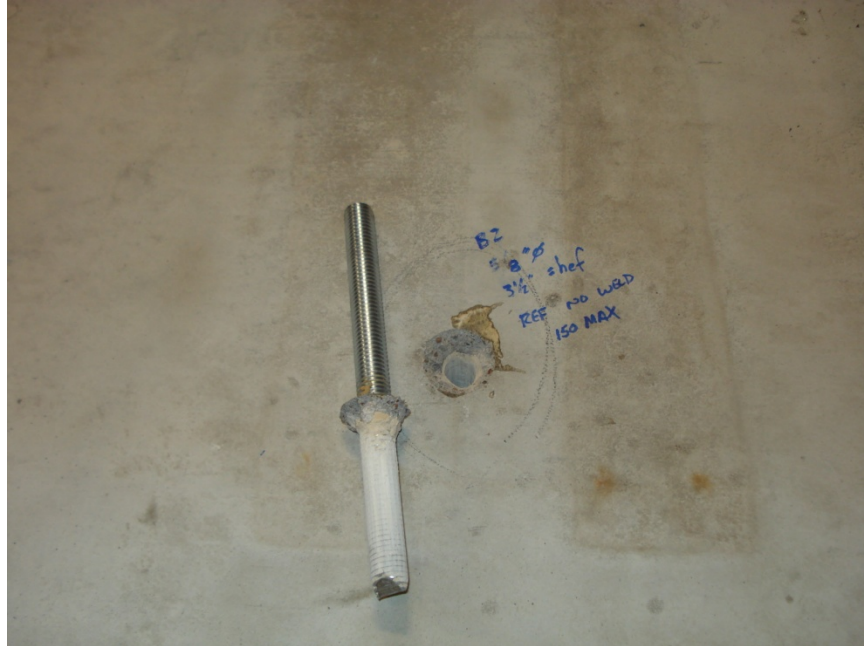
Figure 43: Mixed Bond Failure of Test Group I Reference Test
