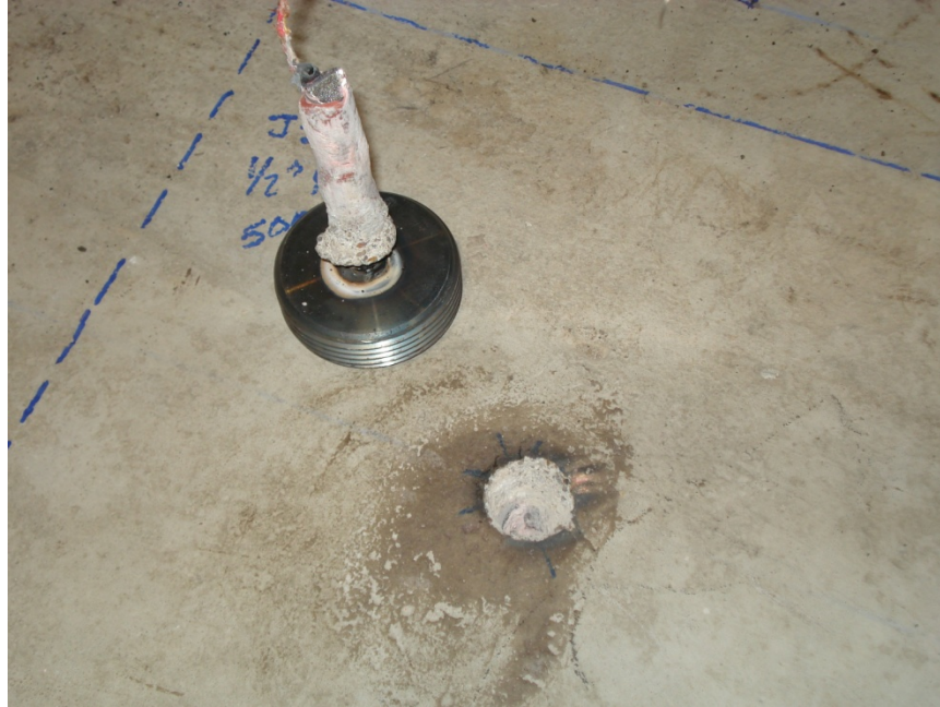
Figure 52: Bond/Borehole Failure of Test Group L Welded Test
