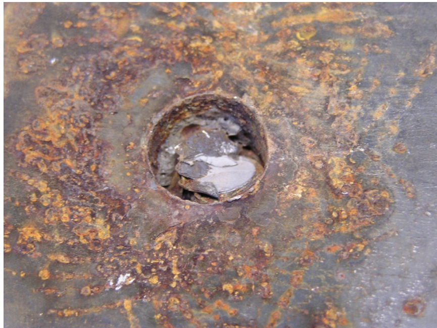
Figure 73: Test Group A Steel Anchor Element Failure Plane near the Root Weld Plane
