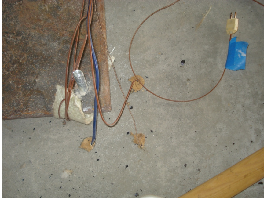
Figure 28: Protective Material Placed between Base Plate and Thermocouple Wires
