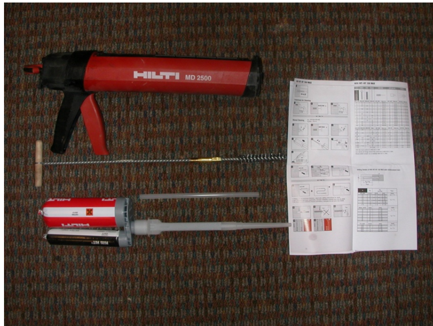
Figure 8: Common Adhesive Anchor System Components
