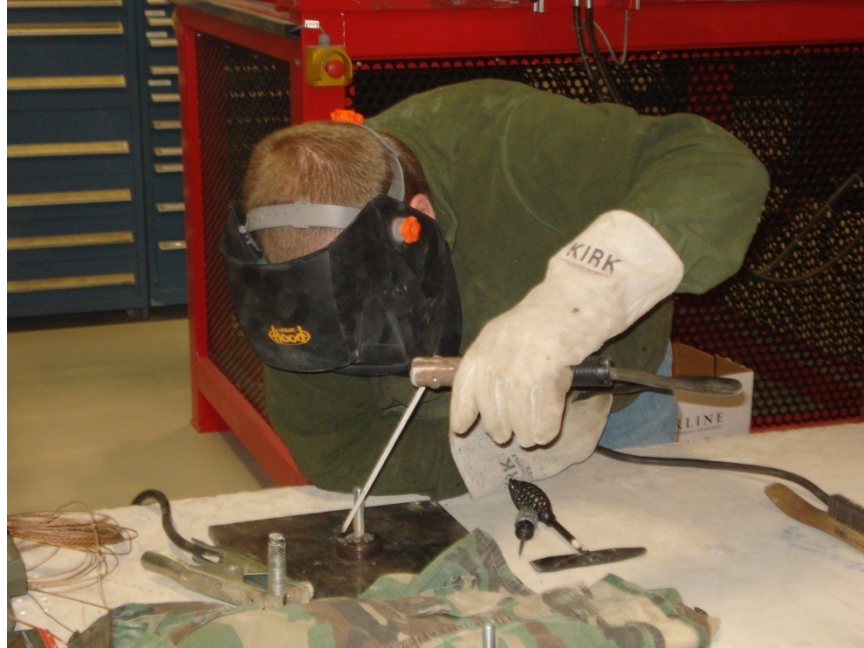
Figure 36: Welding of Anchor to Tensile Fixture
