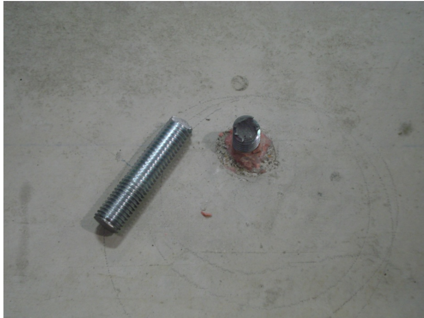
Figure 53: Steel Anchor Element Failure of Test Group M Reference Test
