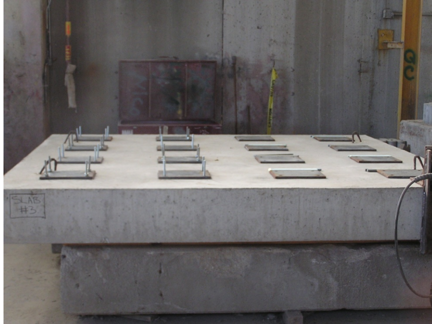
Figure 17: Layout of Eccentric Shear Test Specimens Prior to Stiffened Seat Installation
