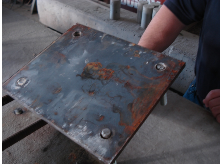
Figure 86: View of Bottom of Base Plate Showing Steel Anchor Element Failure Plane of Test Group C
