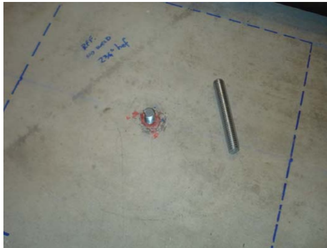
Figure 50: Steel Anchor Element Failure of Test Group L Reference Test
