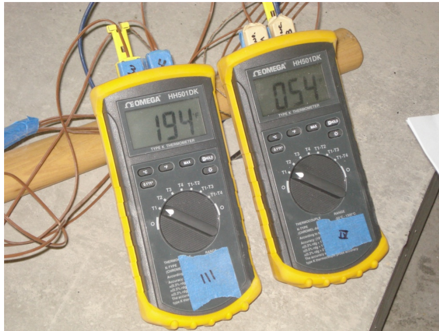
Figure 27: Handheld Thermocouple Thermometers used to Record Weld Temperatures
