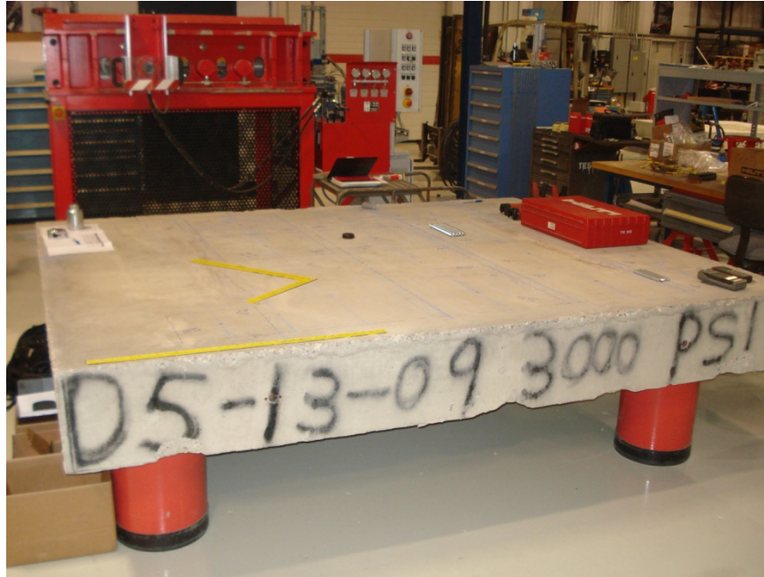
Figure 30: Typical Slab Profile used for Confined Static Tension Tests
