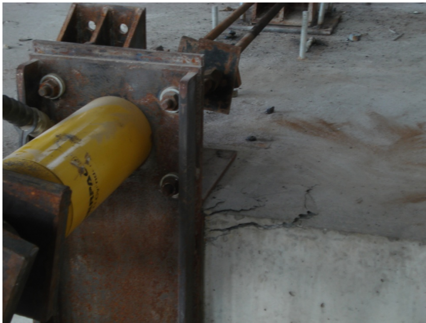
Figure 81: Spall at Edge of Concrete Slab Experienced by Test One of Test Group C
