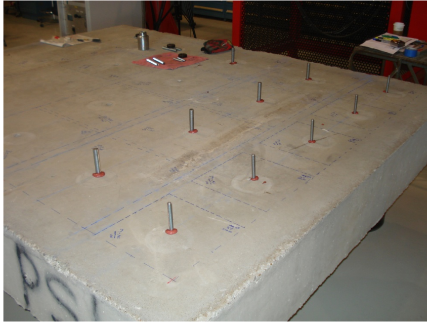
Figure 31: Reference Test Specimens Installed Prior to Testing
