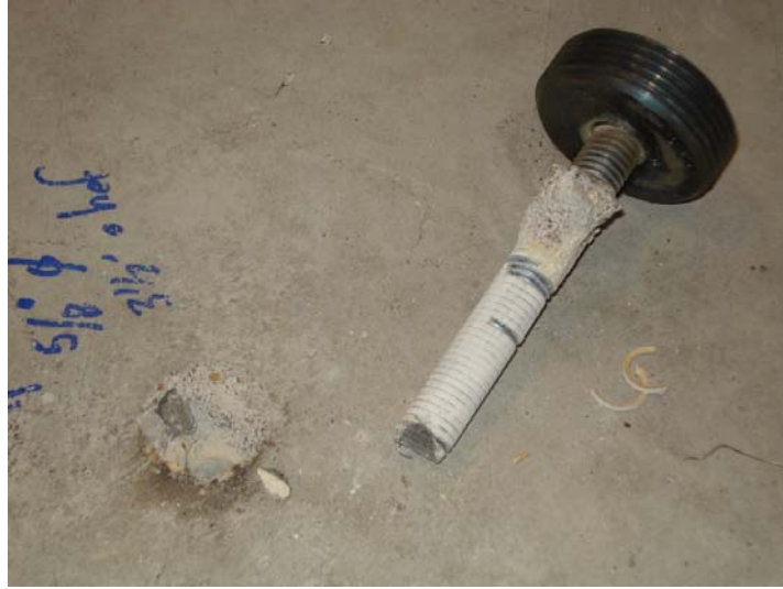
Figure 47: Bond/Element Failure of Test Group K Welded Test
