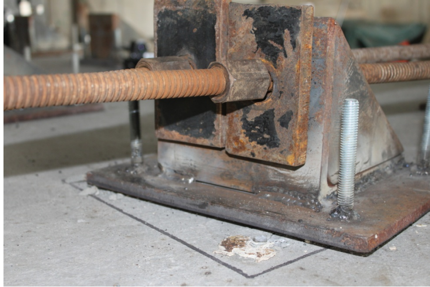
Figure 70: Test Group A Shear and Tension Failure of Two Top (Load Side) Steel Anchor Elements
