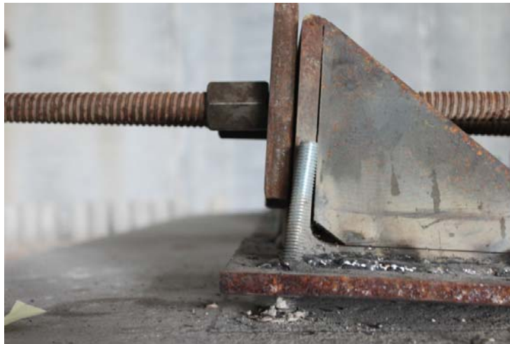
Figure 68: Typical Weld Failure between Test Group A Steel Anchor Elements and Base Plate
