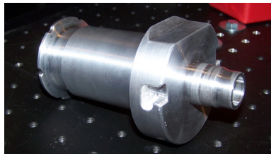
Figure 4.2 An image of the cyclotron adapter flange.
