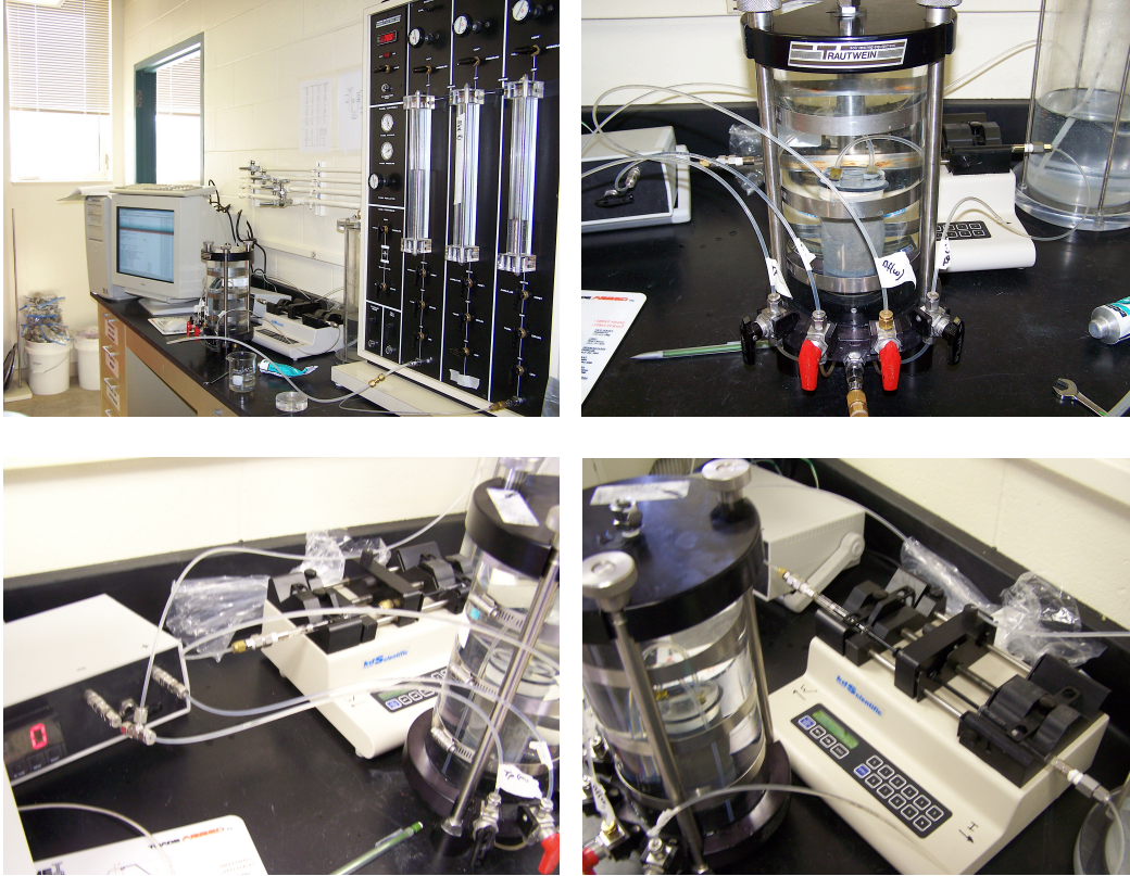
Figure 17. Pictures of constant-flow permeability testing system at University of Missouri-Columbia.
