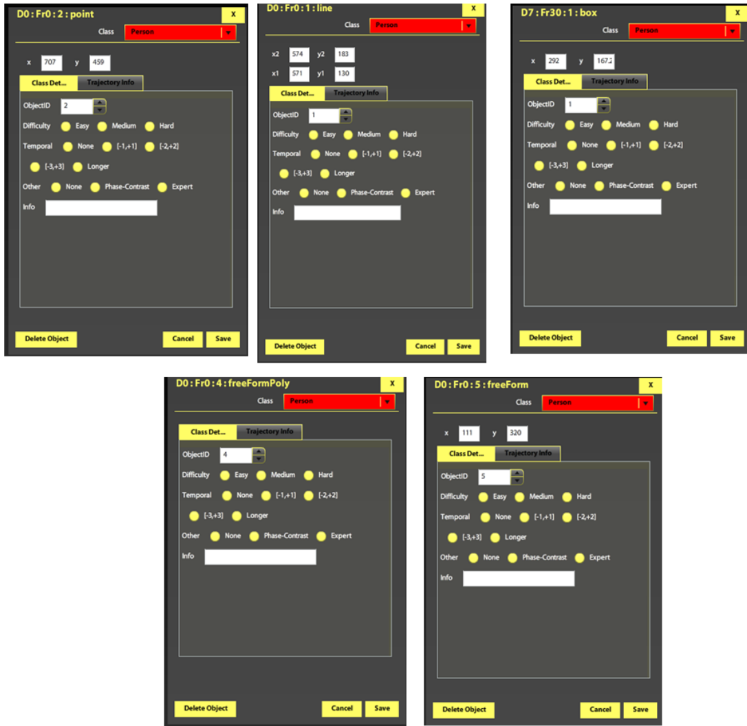
Figure 3.5: Attribute panel for different objects including point, box, line, polyline and polygon
