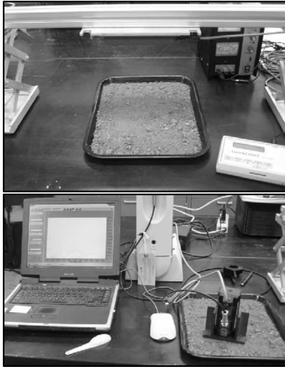
Figure 4.2. Lab set-up of two-band sensor (top) and spectrometer (bottom).
