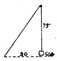
22. In bracing a telephone pole on a corner it is necessary to carry the brace wire across the street to a second pole as is shown in the figure. The second pole is then braced with a second
