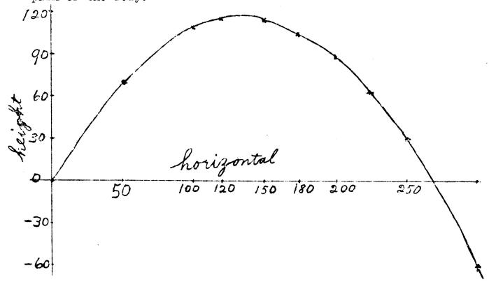
26. Determine from the figure the highest point that the reaches and how many seconds it takes it to reach it. If the body is thrown on level ground how far does it go horizontally? How man seconds before it reaches the ground?
