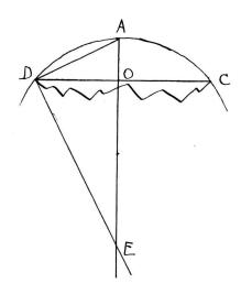
Given segment of water wheel, or water tank, to find the diameter. Let ADC be the segment, to find the diameter AE.
