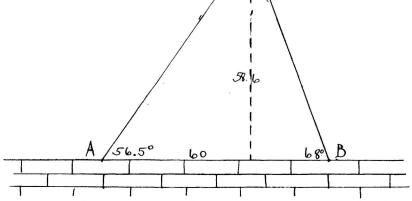
Given the sidewalk AB and a tree C, on the opposite side of the street. To find the width of the street.
