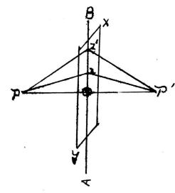
Siven-mirror XY and object P whose image is P'each p'appearing to be equally distant from XY. To prove - XY is the locus of
