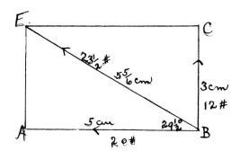
Let AB be 5 cm. (1 cm, = 4#) and AC be 3 cm. Draw AC perpendicular to AB. Complete parallelogram ACDB; and draw diagonal AD; measuring we find AD equal to 5 5/6 cm. Then the resultant will be 23 1/2 pounds. Proof verified by using the dynanometers. The direction is determined by the angle between one of the forces and the resultant, which can be measured with the protractor, and is found to be 29 1/2 degrees. See angle 1.
