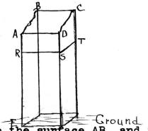
To draw a line RS on the surface AB, and ST on the surface DT as a guide for the saw.
