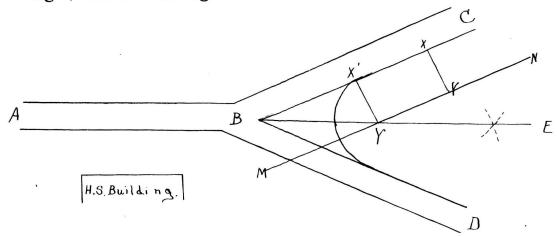
Given: the streets AB, BC and BD. To find line of front of building of 60 foot radius. Bisect the angle DBC with line BE. Erect perpendiqular XY to BC and lay off distance equal to 60 feet, and at Y draw MN perpendicular to XY at Y. The point of intersection of MN and BE will be the centre of the circle, that will be tangent to the streets, with radius 60 feet. This meets the requirements 60 feet from the streets and also equal distant from each street.
