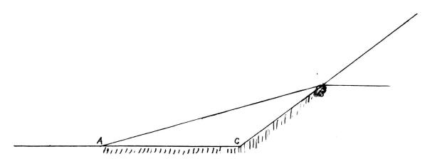
Select a point C at the foot of the embandement lying in the same vertical plane as a and B, and measure the distances all and CB and the angle Bal. By an easurement find BC equal to 36 feet and acc = 32 & feet and angle aCB on protractor is 141 degrees. Construct straight line acc 32½ ann. long and with protractor construct angle aCB, 141 degrees. Braw BC = 36 ann. all and analying the distance ab equal to 65½ feet.
