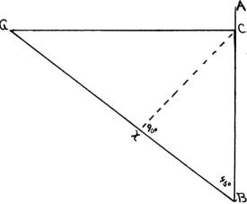
Given: a lighthouse A and a ship amoving along aB in the direction of BC. The distance from the light house at which the ship passes the light house is found by noting the anoment the ship makes an angle of 45° with the light house or the (CBC and also the time the ship makes an angle of 90° with the light house or (CXB.
