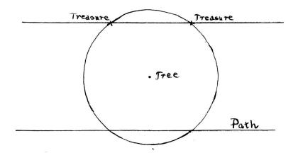
If the treasure is 75 feet from a certain tree, it must lie on the circumference of a circle whose radius is 75 feet. If 100 feet from a path it must lie on a line parallel to the path at a distance of 100 feet. There are two, one or no solutions depending upon whether the circumference cuts the straight line in two points, or whether it is tangent to it or whether it lies entirely outside of its field.
