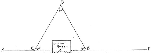
Suppose A to be the school house and BCEF the straight line to be determined. At point C construct angle  $1^1$ = 60 degrees and lay off DC any convenient distance, at least long enough to see beyond the building, and at D construct angle 3 = 60 degrees and draw DE = DC and at E construct angle 2 = 60 degrees, and draw EF. Then BCEF is a straight line, and CE = DC or DE. Distance from B to F is BC plus CD or (DE) plus EF.
