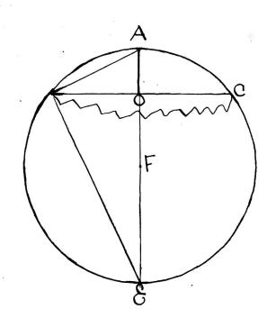
Hiven: a segment of a water wheel (or water tank. Let a DC be the segment. Find: The diameter a E.
