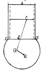
The form of an inverted cup, is 5 inches in inside diameter; the crank aB, 5" between the centers of the pivols; and the connecting rod ac 17" between the centers of the pivols, and the pivols, and the diameter of aC being 1".
