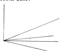
Set a vertical post. From ten in the morning until two in the evening take readings every fifteen minutes. The readings are the lenghts of the shadows. At night determine a north south line through the foot of your perpendicular post by means of the North Star. Verify this line with a compass. Then with a protractor draw an east west line. Verify this with a compass.
