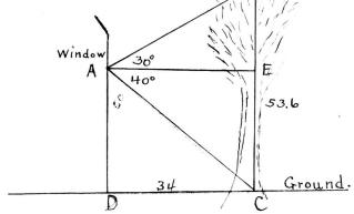
Given: a tree at a distance of 34 feet from the building. To find the height of the tree.
