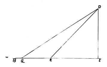
Take any point near the school building from which the top of the building can be seen and sight to the top of the building. With a proteastor the angle formed by the line sighted to the top of the building and the ground is measured and found to be 47? From this point, C, measure off any convenient length as so ft. at the end of this line, a, sight to the top of the building. This angle is found to be 33.5?
