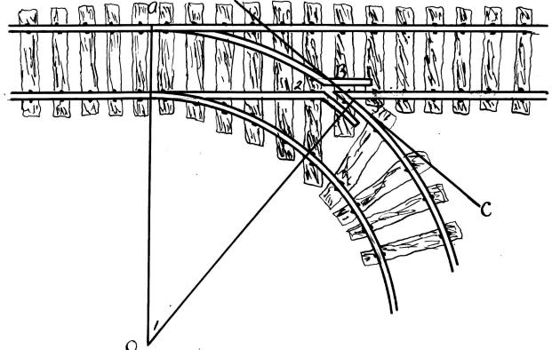
From from t O draw radii O a and O B. The central angle 1 is measured by arc asses. Angle 2 is measured by 2 arc asses. Therefore these two angles are equal. The verticle angles 2 and 3 are equal. Therefore angle 1 equals angle 3. Magnatudes which are equal to the same magnitudes or equal magnatudes are equal to each other!
