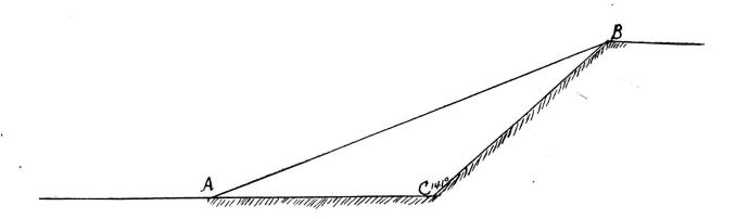
Select a point C at the foot of the embankment lying in the same vertical plane as A and B, and measure the distances AC and CB and the angle BAC. By measurement find BC equal to 36 feet and AC equal to 32 1/2 feet and angle ACB on protractor is 141 degrees. Construct straight line AC 32 1/2 mm. long and with protractor construct angle ACB, 141 degrees. Draw BC = 36 mm. AB measures 65 1/2 mm. making the distance AB equal to 65 1/2 feet.
