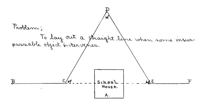
Suppose a to be the school-house and BCEF the straight line to be determined. at point a construct ungle! = 60 degrees and lay off DC any convenient distance, dt least long enough to see by the building, and at he construct angle 3 = 60 degrees and draw HE = HC and at E construct angle 2 = 60 degrees, and draw EF. Then BCEF is a straight line, and CE = HC or HE. Distance from B to F is BC plus CIO m ME. CD or (DE) plus EF.
