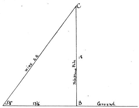
Draw a straight line AB 13 1/2 (1/2 cm,) long and at B<sup>1</sup> erect a perpendicular CB and measure on CB the distance 18 (1/2 cm,) Then draw AC. Measure AC and find it to be 22 (1/2 cm.), hence the wire is 22 feet long. Measuring the angle CAB with a protractor it is equal to 58 degrees.
