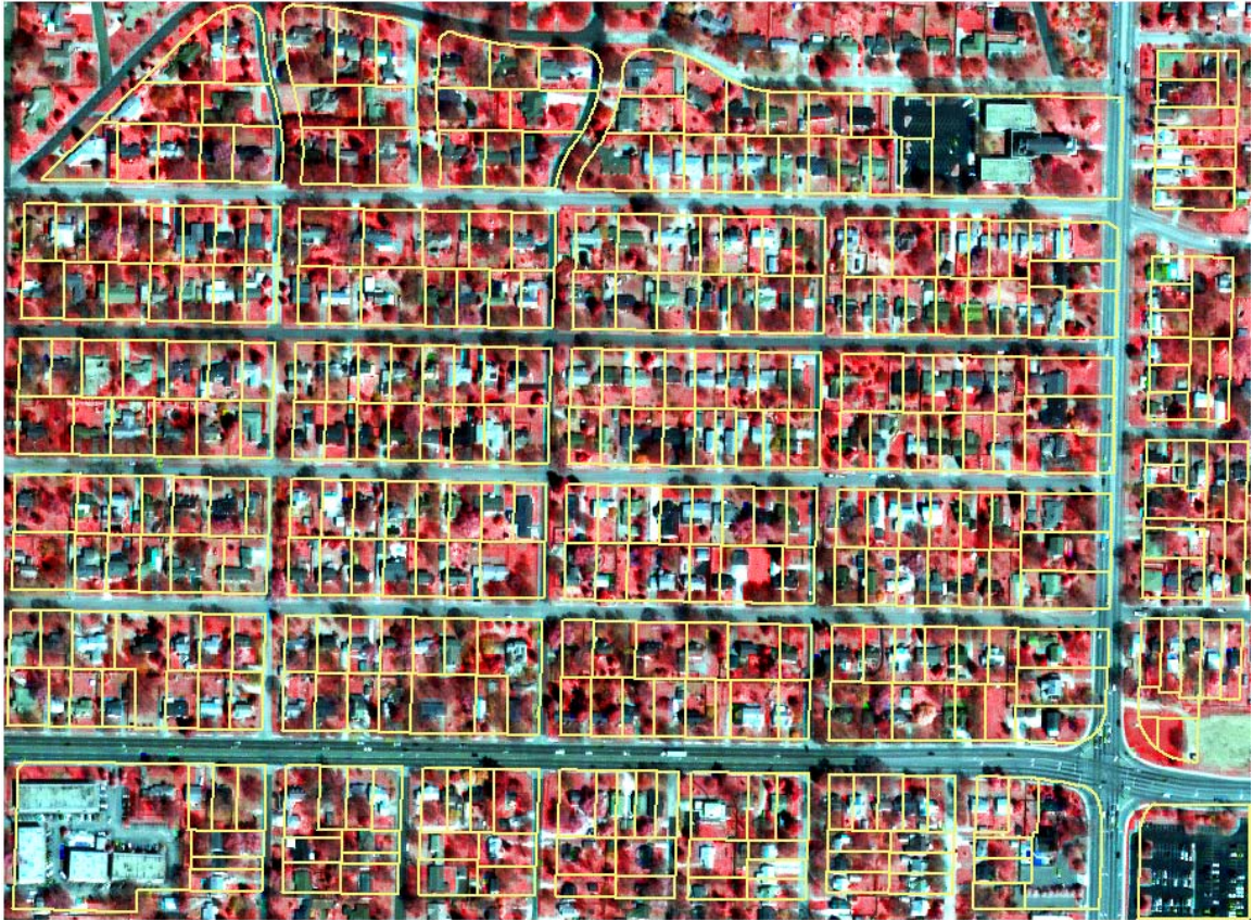
Figure 6.3 Original parcel lines (yellow) overlaid on the high-resolution IKONOS imagery. It is obvious that many parcel lines cut through houses.
