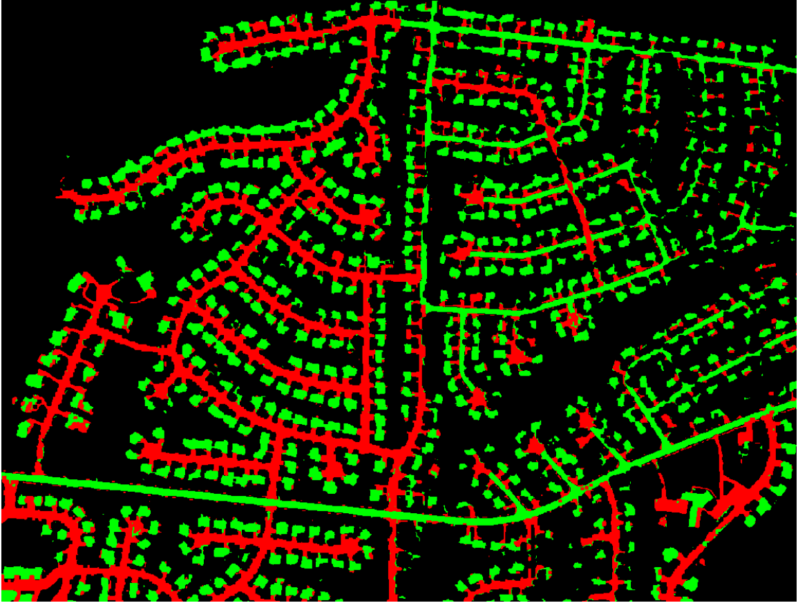
Figure 5.10 The classification results. Bright roads are red. Darker roads and buildings are green. Black are non-road class.
