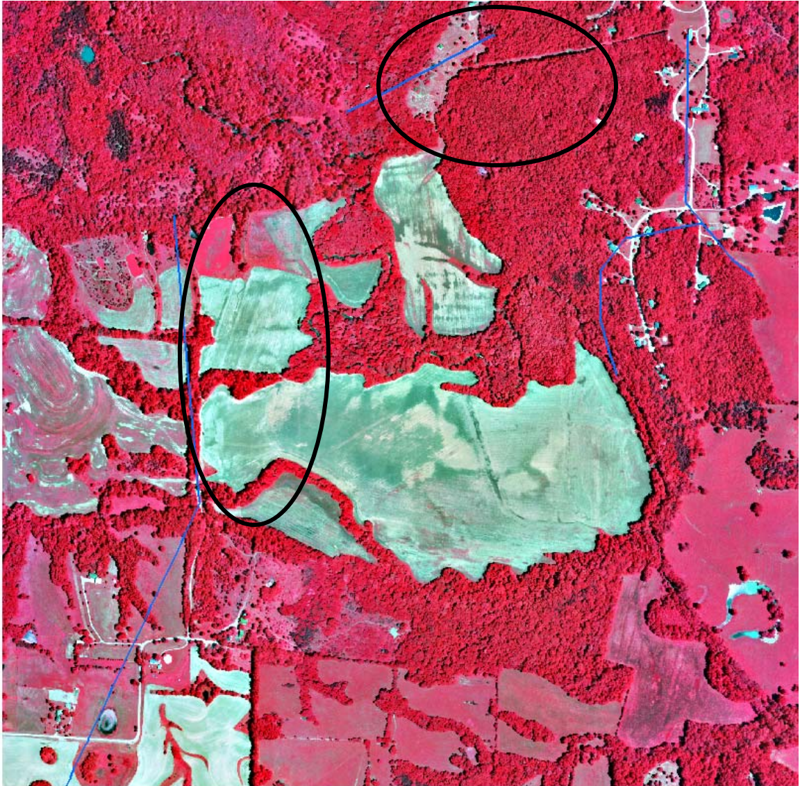
Figure 5.14 The TIGER roads are overlaid on imagery. The road segments within the black oval are errors. Actually they do not exist.
