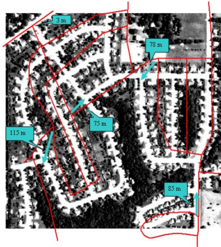
Figure 4.1 The TIGER vector roads (red) are superimposed on an aerial photograph. The non-systematic discrepancy ranges from a few meters to over 100 meters, and has diverse directions.
