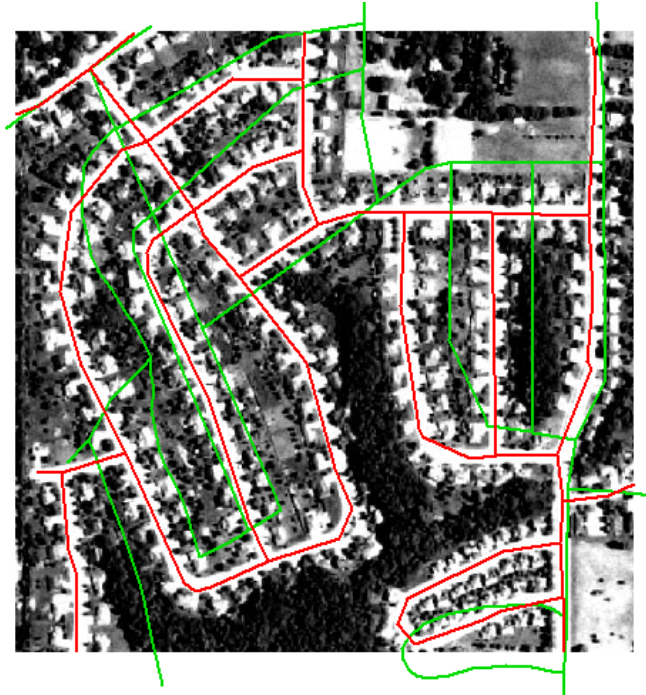
Figure 4.3 Comparison of original TIGER roads (green) and final conflation result (red) for test area shown in Fig. 4.1
