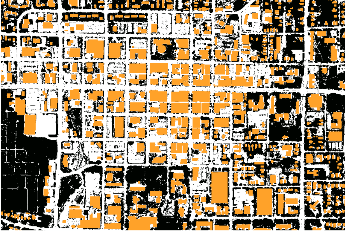
Figure 5.29 The vector building footprints (yellow polygons) are used as mask to clip out buildings from road image.
