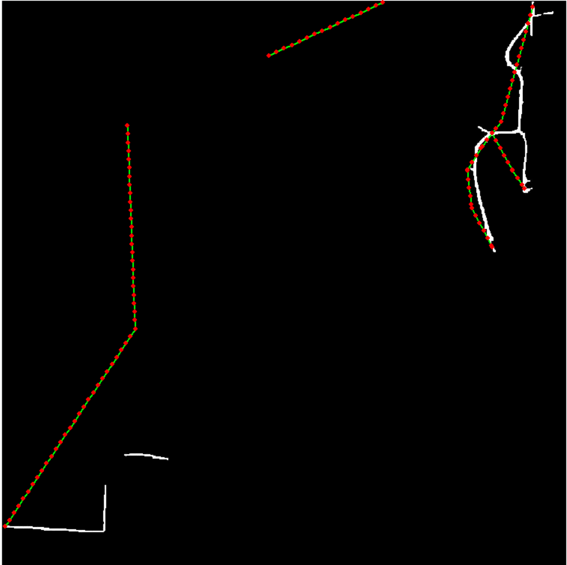
Test area Rural_01. The rubber-sheeting adjusted TIGER roads (green) with vertices (red dot) are overlaid on road imagery.
