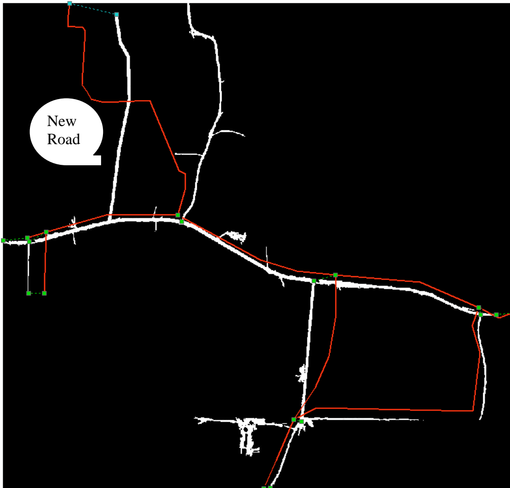
Figure 5.24 Original TIGER roads (red) in test area Urban07 are overlaid on the road mask with an additional road edited in to demonstrate a limitation of a fully automated approach. The green dashed lines indicate the matched road intersections found by relaxation labeling algorithm.
