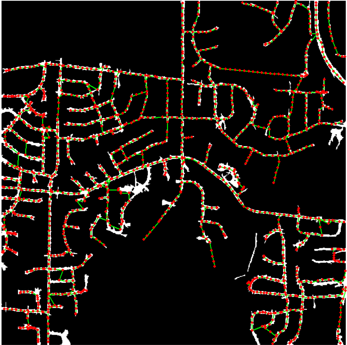
Test area Urban_09. The final conflated TIGER roads (green) with vertices (red dot) are overlaid on road imagery.
