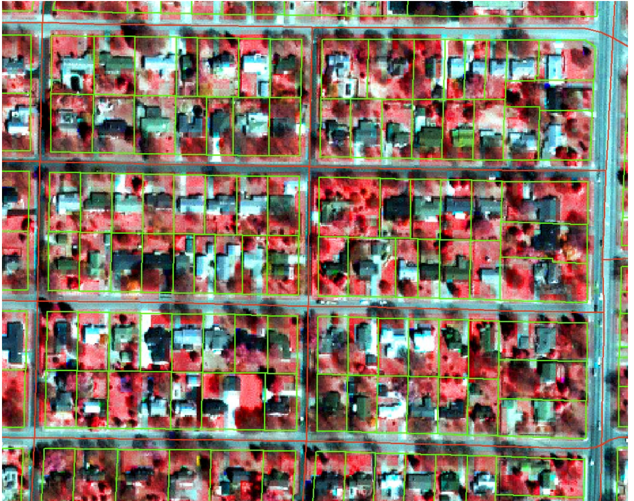
Figure 6.8 Zoom-in section of the parcel lines (green) and road centerlines (red) after vector-to-imagery conflation
