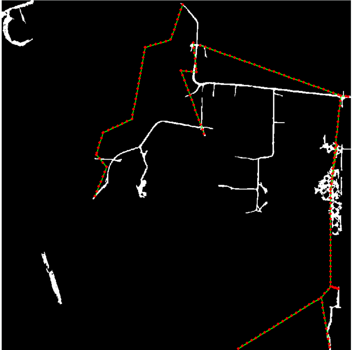
Test area Rural_04. The rubber-sheeting adjusted TIGER roads (green) with vertices (red dot) are overlaid on road imagery.
