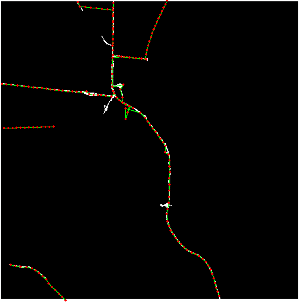
Test area Rural_05. The final conflated TIGER roads (green) with vertices (red dot) are overlaid on road imagery.
