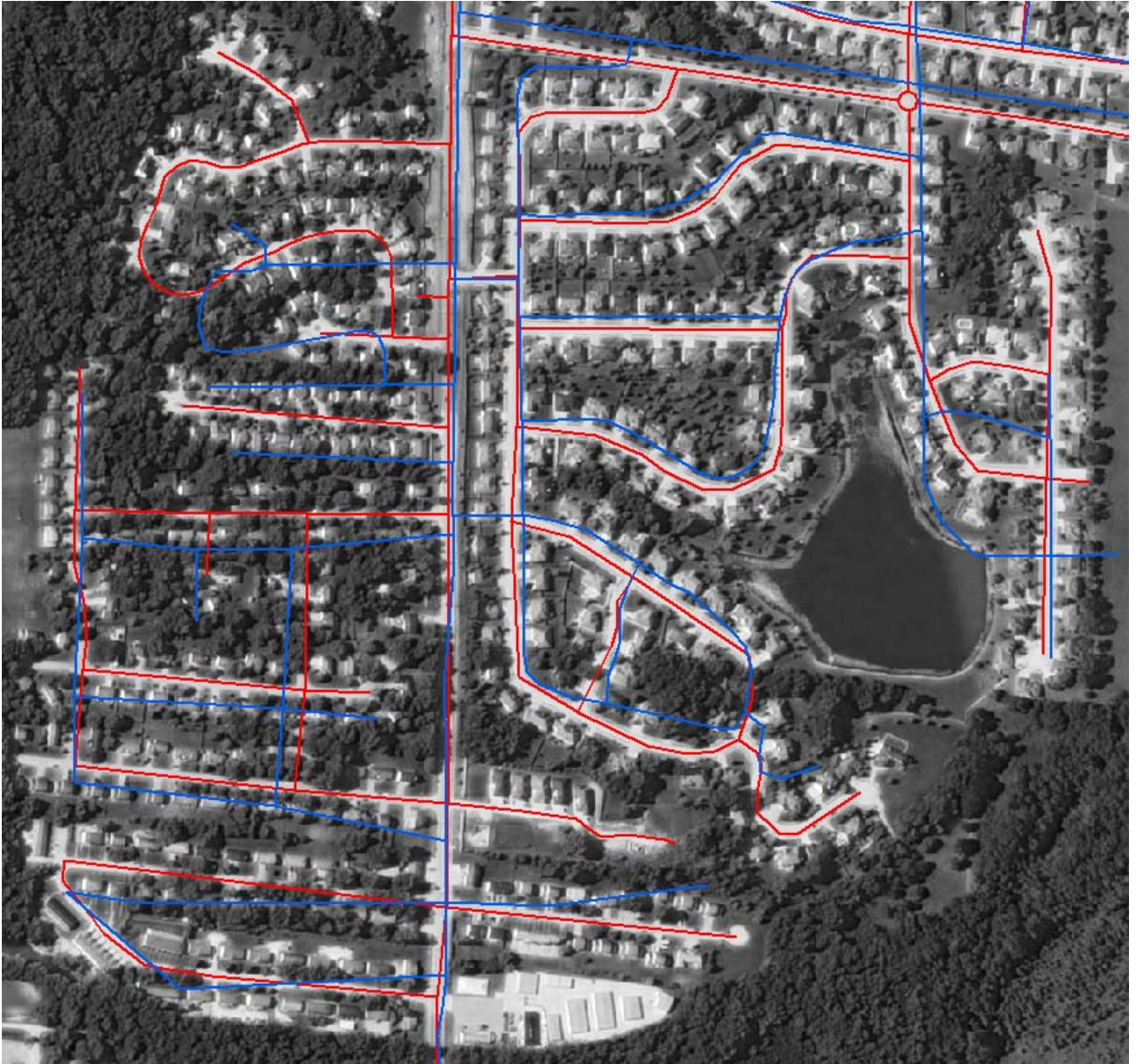
Figure 3.1 TIGER roads (blue) and MODOT roads (red) are superimposed on an aerial photograph. The nonsystematic discrepancy problem between the two datasets is easy to see.
