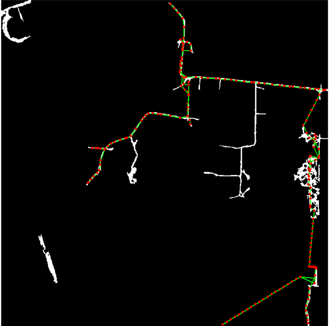
Test area Rural_04. The final conflated TIGER roads (green) with vertices (red dot) are overlaid on road imagery.
