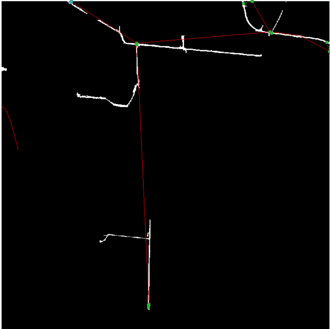
Test area Rural_02. Original TIGER roads (red) are overlaid on road imagery. The green dashed lines indicate the matched road intersections found by relaxation labeling algorithm.
