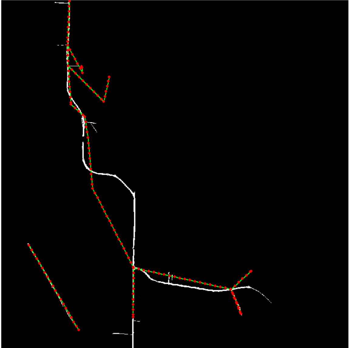
Test area Rural_08. The rubber-sheeting adjusted TIGER roads (green) with vertices (red dot) are overlaid on road imagery.
