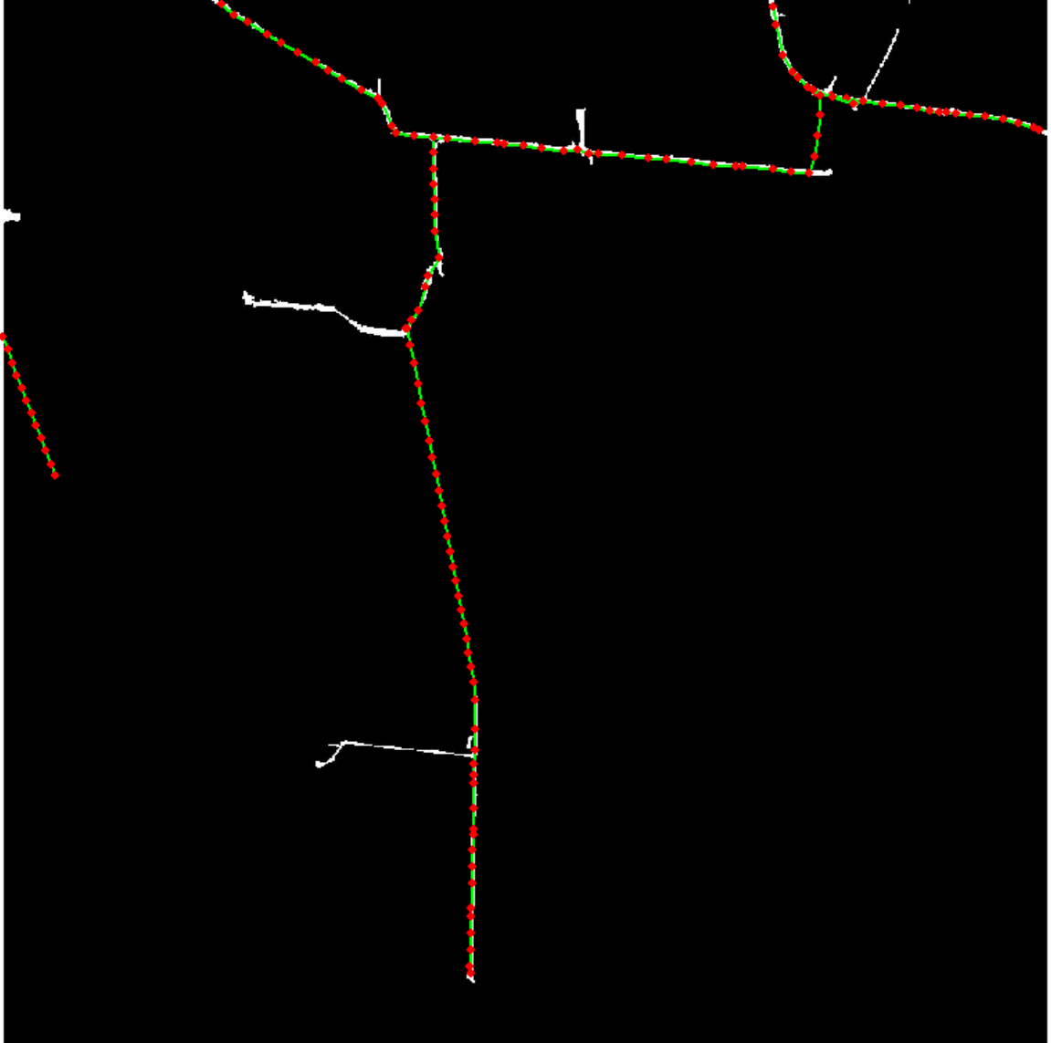
Test area Rural_02. The final conflated TIGER roads (green) with vertices (red dot) are overlaid on road imagery.
