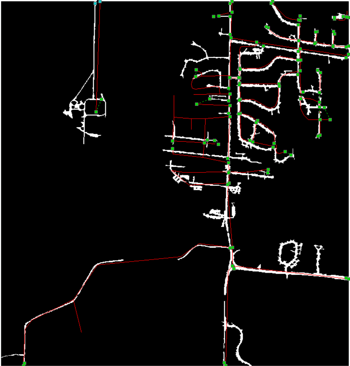
Test area Urban_05. Original TIGER roads (red) are overlaid on road imagery. The green dashed lines indicate the matched road intersections found by relaxation labeling algorithm.
