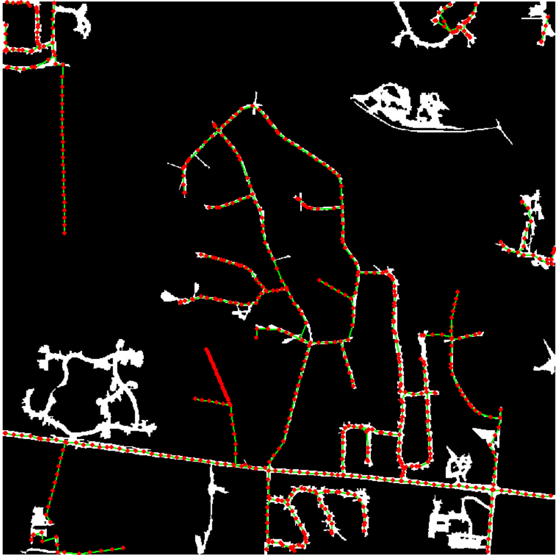
Test area Urban_06. The final conflated TIGER roads (green) with vertices (red dot) are overlaid on road imagery.
