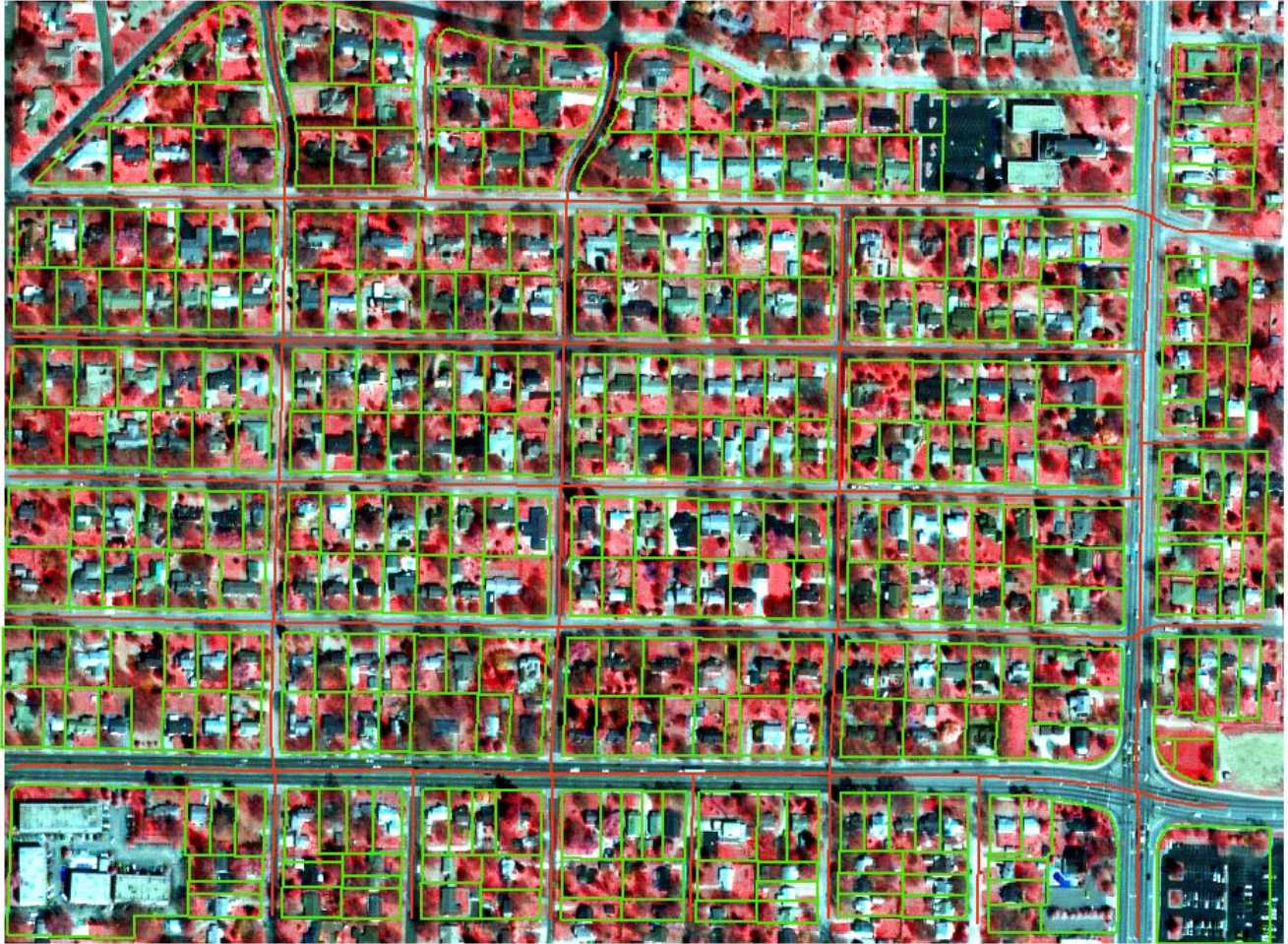
Figure 6.7 after running vector-to-imagery conflation, the adjusted parcels (green) and road centerlines (red) are in line with imagery.
