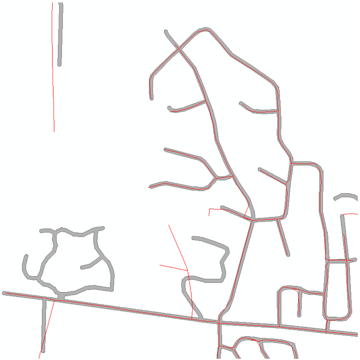
Figure 5.16 The conflated TIGER roads are overlaid on buffer zone generated from MODOT roads.
