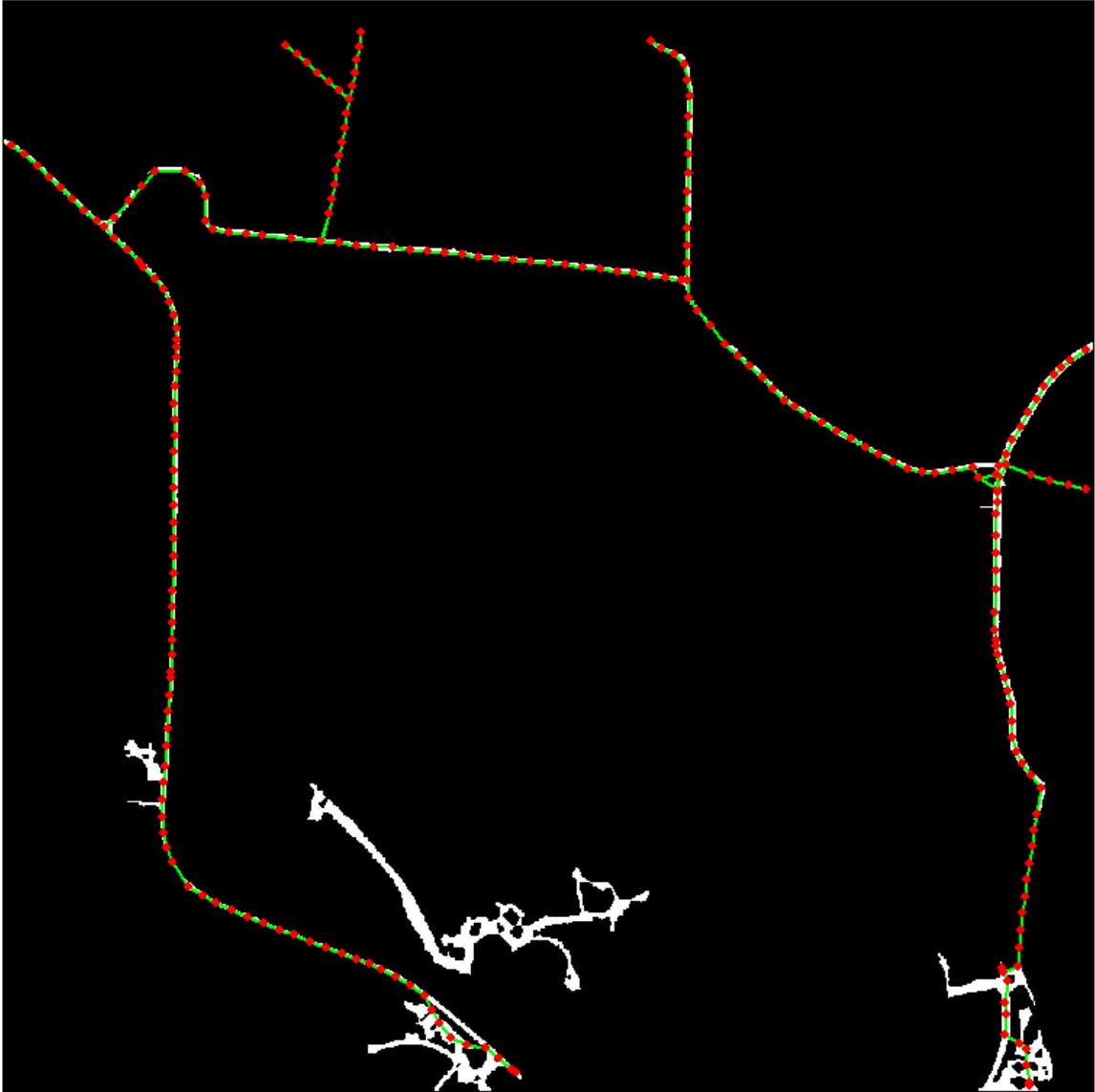
Test area Rural_03. The final conflated TIGER roads (green) with vertices (red dot) are overlaid on road imagery.
