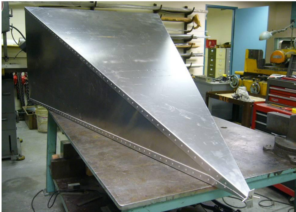
Figure 4 - 10 The constructed tapered transmission section.
