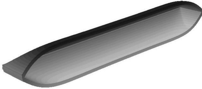
Figure 52. Exaggerated deflection of fully constrained boundary condition simulation
