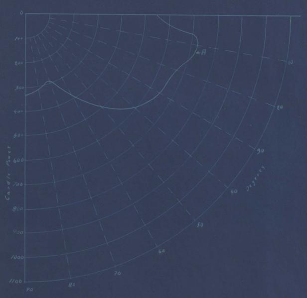
A -- 4 Amp D.C. Magnetite Arc Lamp
