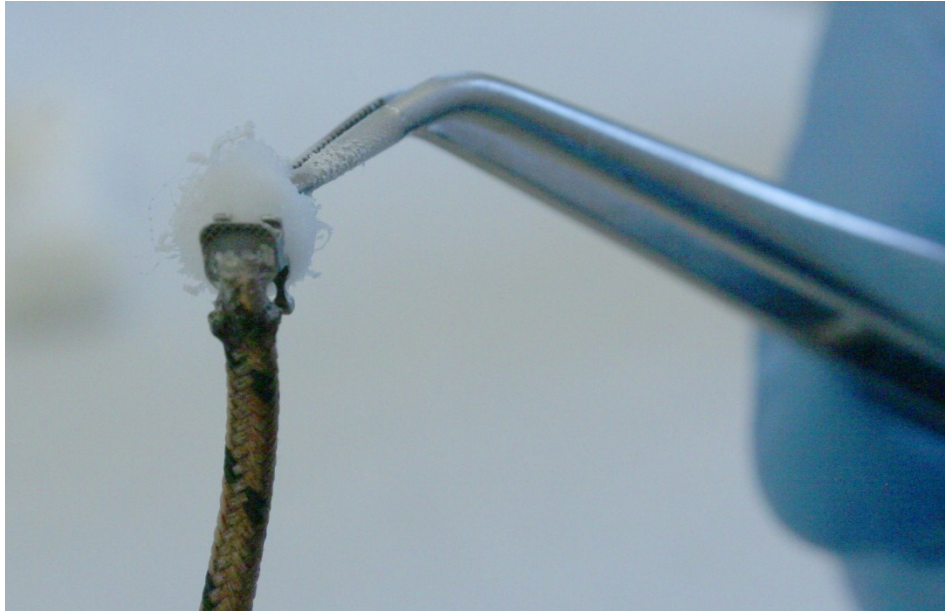
Figure 5. Thermocouple Attached to Cured Composite for Composite Temperature Testing. A bracket with composite cured on the bracket base. A k-type thermocouple is attached to the composite layer in order to record the temperature of the composite layer during a 15 s application time of refrigerant spray delivered to the bracket via a cotton pellet using forceps.
