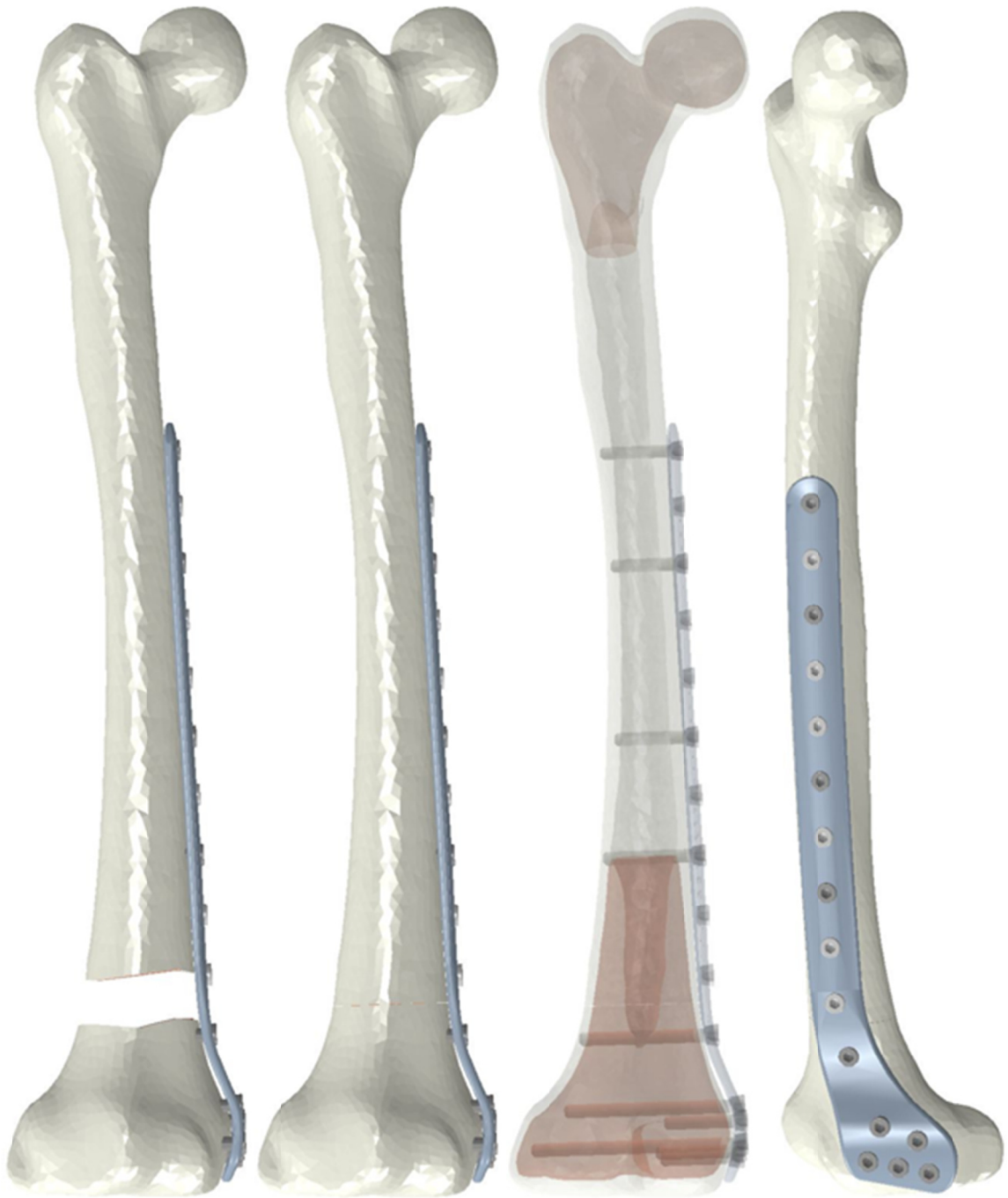
Fig. 102. Fracture model using the optimized MLP ( far left: fracture with bone loss, right three: distal fracture )
