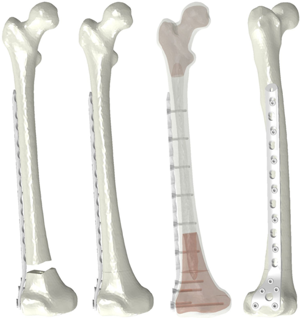
Fig. 65. Fracture model using Synthes LCP ( far left: fracture with bone loss, right three: distal transverse fracture )
