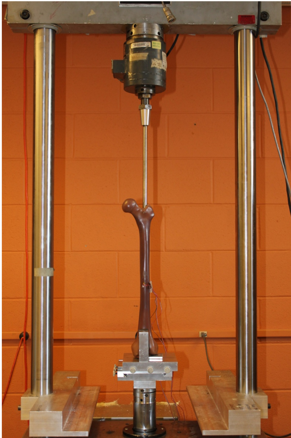
Fig. 36. Experimental setup: MTS universal testing machine with femur fixture, Sawbones composite femur, and prototype IM nail
