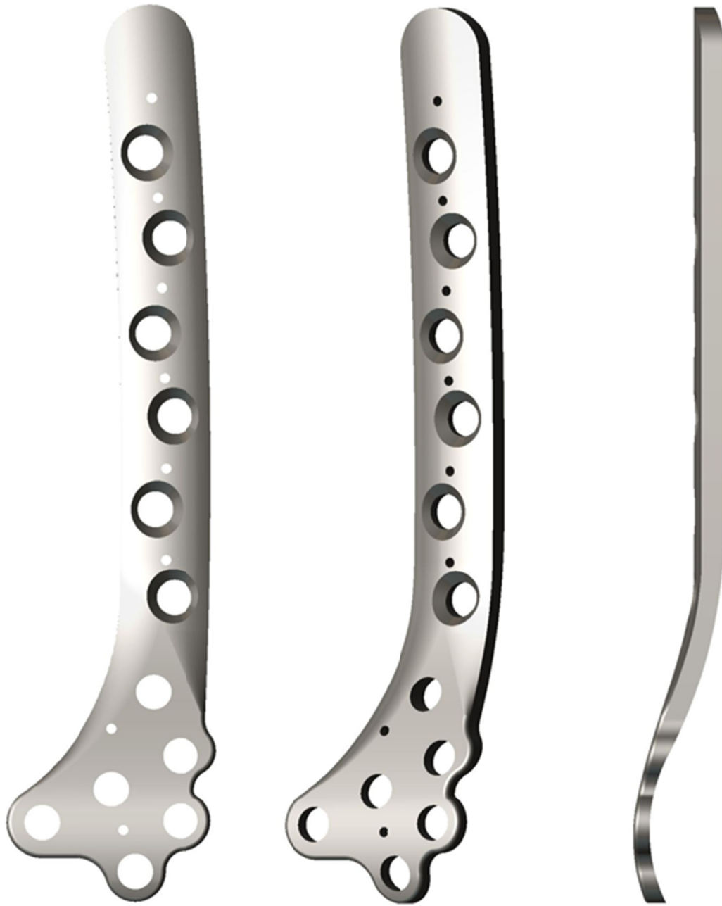
Fig. 59. CAD model of Smith & Nephew PERI-LOC plate
