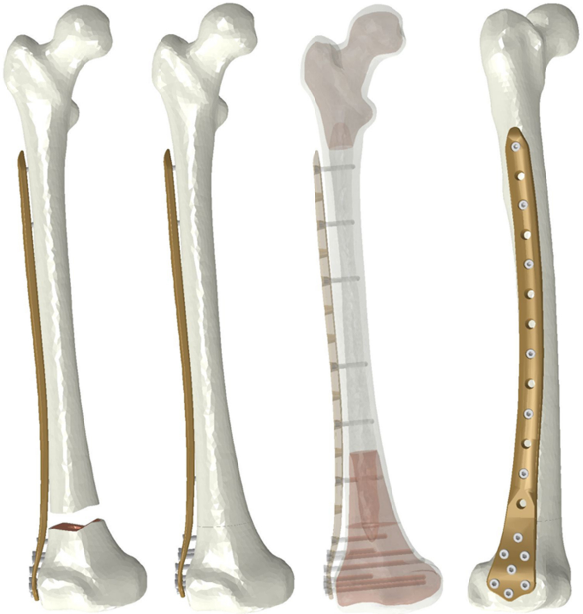
Fig. 66. Fracture model using Synthes LISS ( far left: fracture with bone loss, right three: distal transverse fracture )
