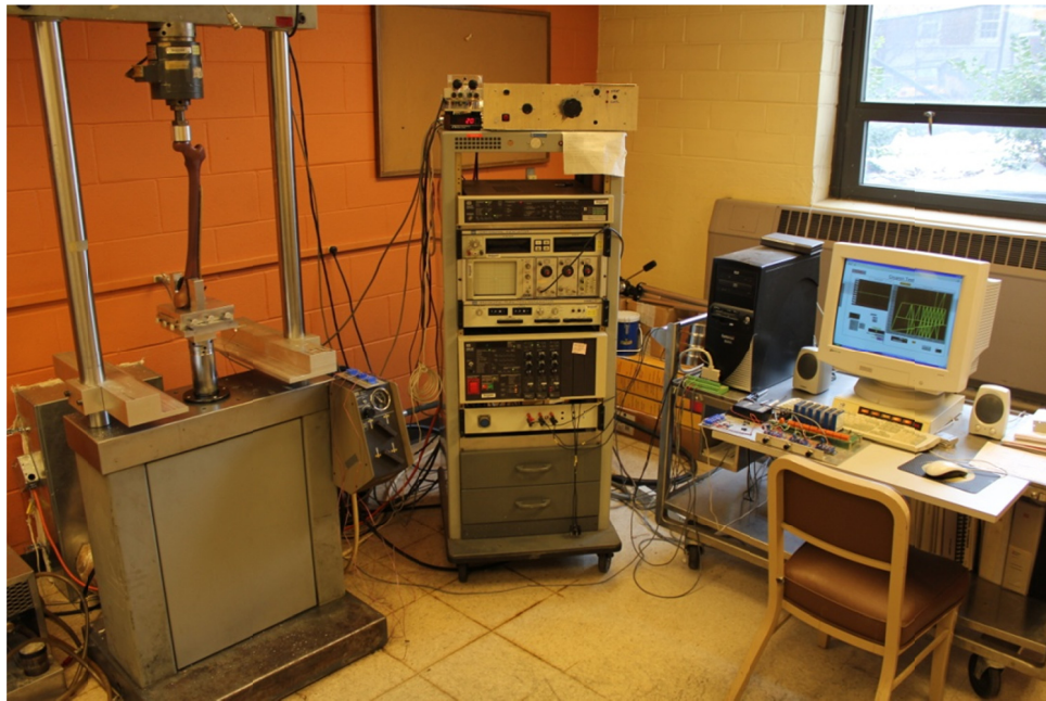
Fig. 77. Experimental setup of MTS Universal Testing Machine
