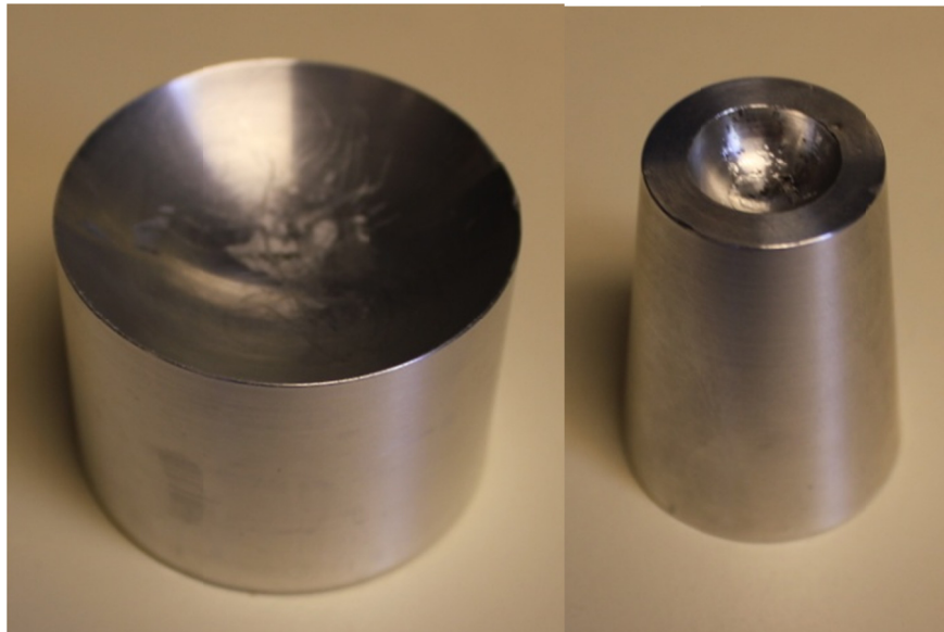
Fig. 12. Proximal femur fixture for MTS universal testing machine ( Left: hip joint fixture, Right: IM nail fixture )
