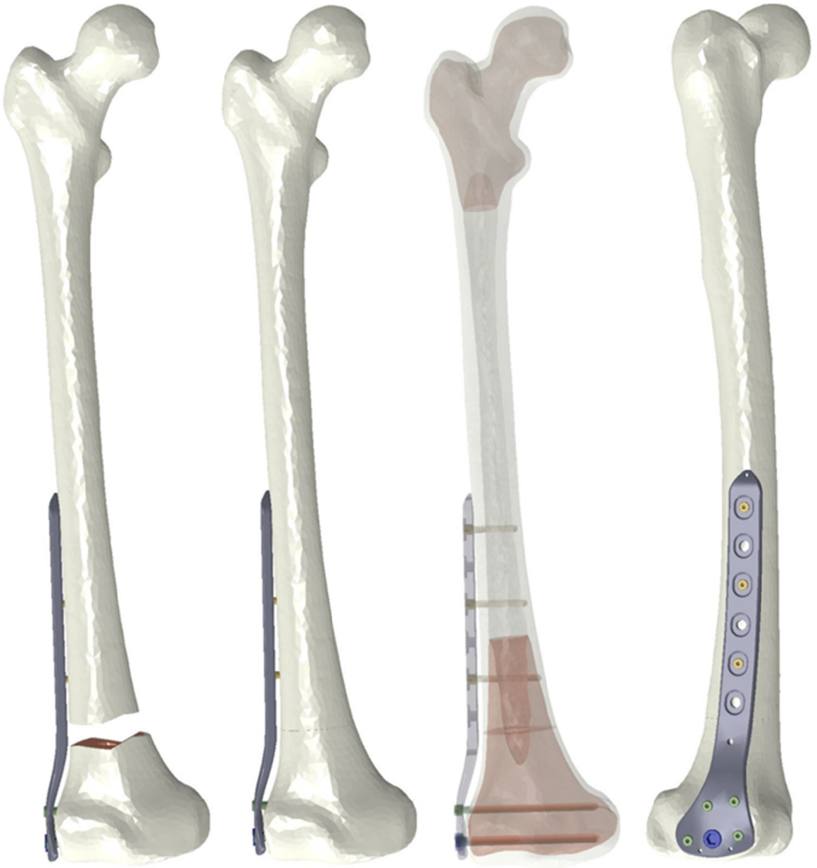
Fig. 63. Fracture model using DePuy POLYAX plate ( far left: fracture with bone loss, right three: distal transverse fracture )
