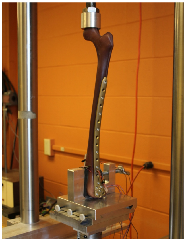
Fig. 81. Experimental testing of intact femur fixated with Synthes LISS
