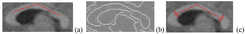
Fig. 2.3. An example of the initialized seed. (a) User-initialized polyline. (b) The edge map. (c) The completed seed contour.
