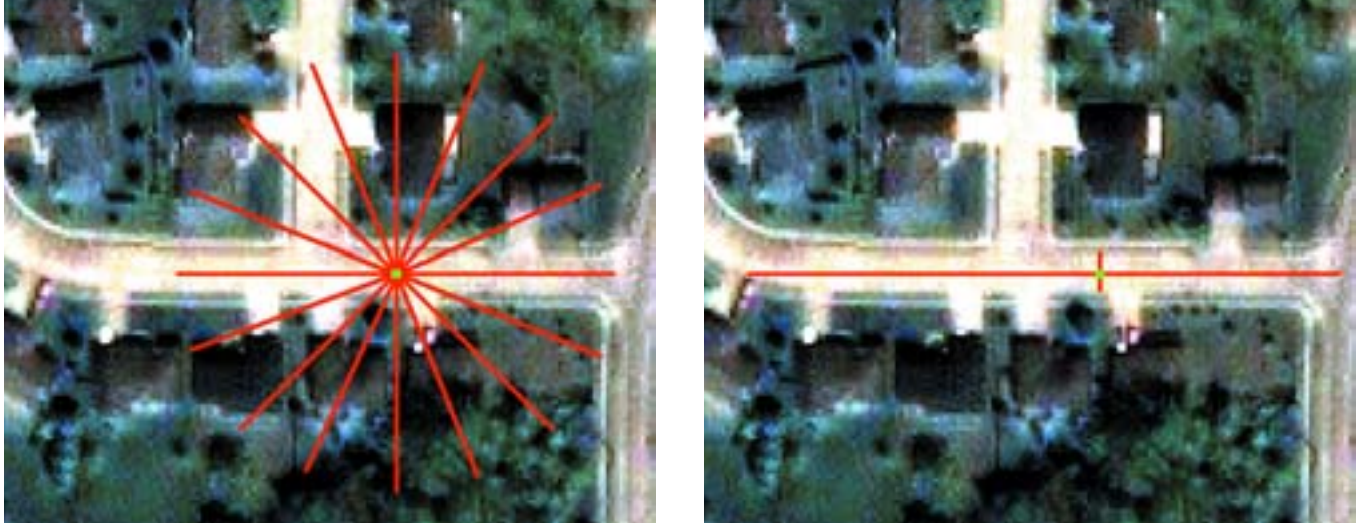
Figure 1 2D spatial signature determination for a single road pixel. Left: line segments radiating out from central pixel are examined for spectral similarity. Right: maximum and minimum length line segments identified.
