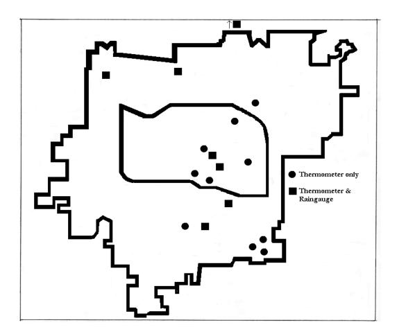
*Figure 1.* The station location and distribution of the temperature and rain gauge network. Closed squares represent the deployment of both thermometers and rain gauges, while closed circles represent the deployment of only one instrument (see legend).
